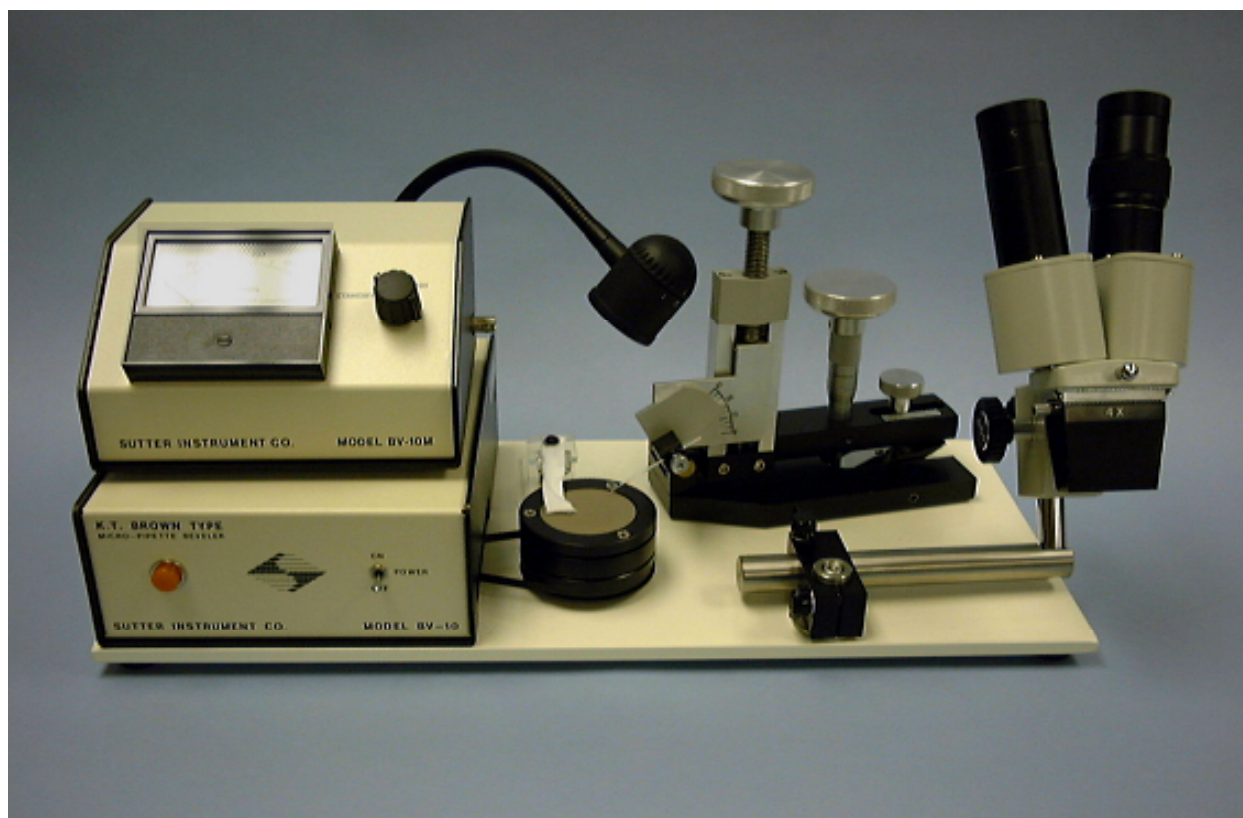
Figure 4. BV-10 beveler component layout.
