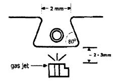
After installing your trough filament, you will need to run a new ramp test to establish the appropriate heat settings.
