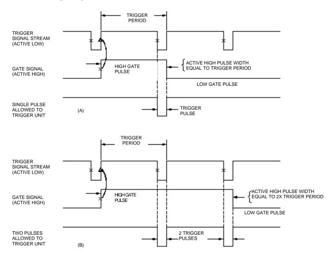
Figure #5A and 5B GATE Input Timing Diagram
