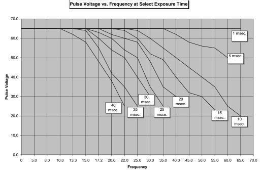
Figure #8 Pulse Voltage vs. Frequency
