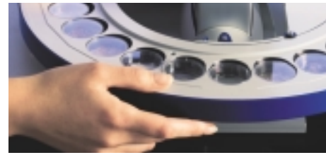
A special click stop mechanism exactly positions each specimen.
