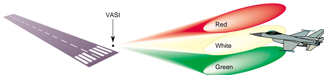
Figure 21-1 VASI Landing Light
