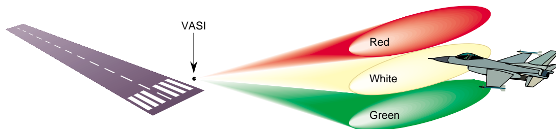
Figure 21-1 VASI Landing Light
