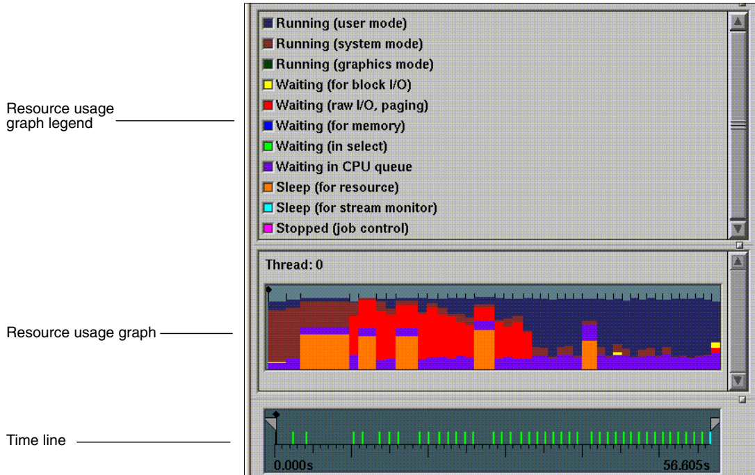
Figure 3-3 Machine Resource Usage in Performance Analyzer Window
