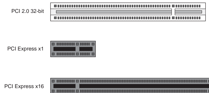
Figure 6-14 Comparison of PCI/PCI-X Connector with PCI Express Connectors
