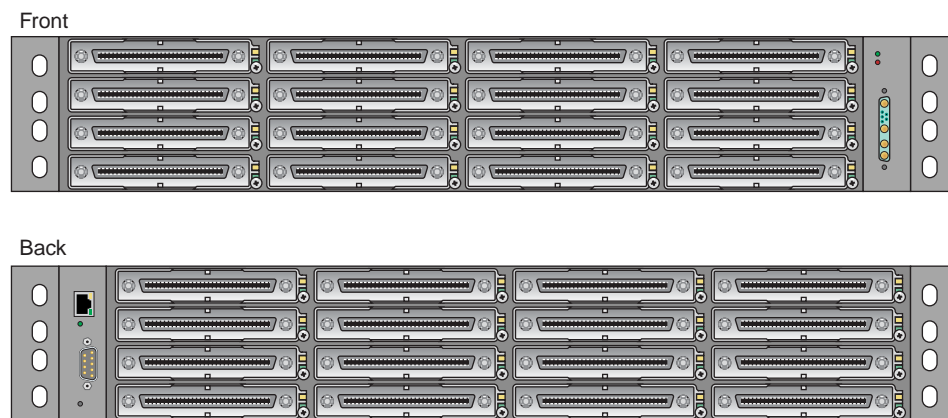
Figure 5-2 Dense Router Module Front and Rear Panels
