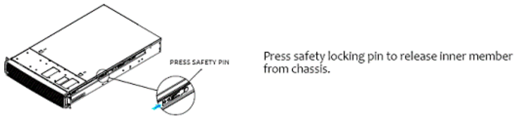
Figure 4-22 Removing the Inner Member from the Chassis
