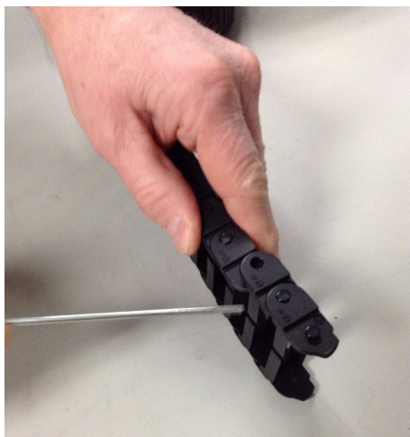
Figure 1-49 Pry the Joint Apart
