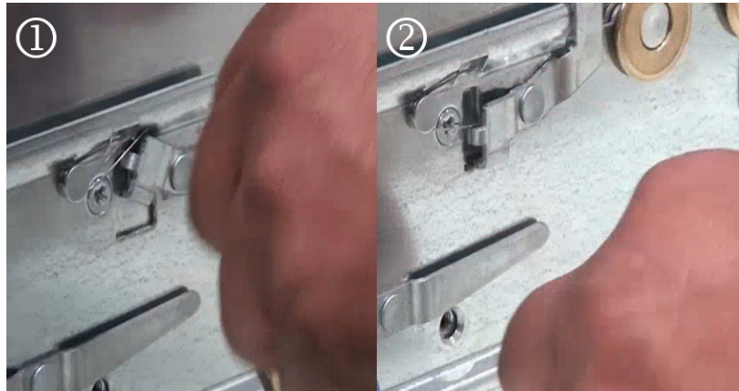
Figure 1-21 Return Latch to Home Position
