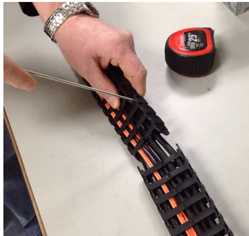
Figure 1-55 Pry Apart the Joint at the Other End
