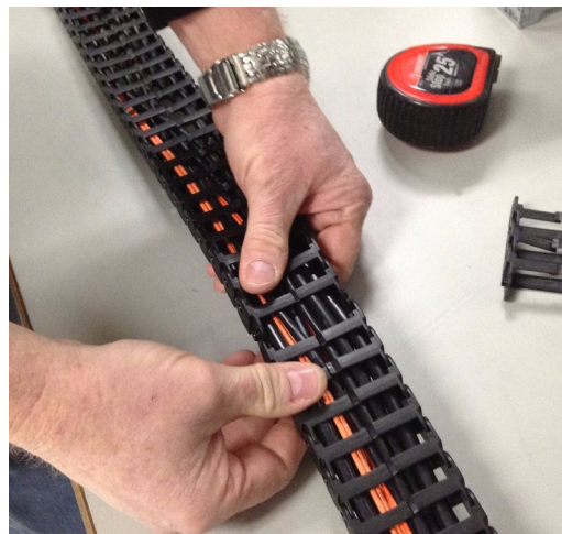
Figure 1-57 Join the Spliced Ends of the Cable Management Arm
