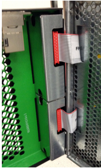
Figure 1-4 Control Panel Ribbon Cables Attached to Front Bezel
