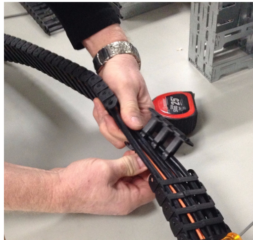
Figure 1-56 Twisting the Section of Segments from the Cables
