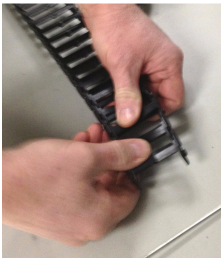
Figure 1-50 Pull the Segments from the Arm
