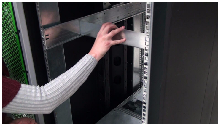
Figure 1-16 Slide the Alignment Tool from Front to Back
