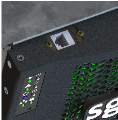
Figure 1-76 MIS-S9D Proprietary Network Interface
