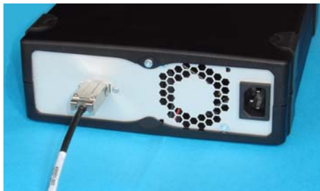
Figure 3 Infiniband type of connector used to connect to a SAS HBA external port (SFF8470)
