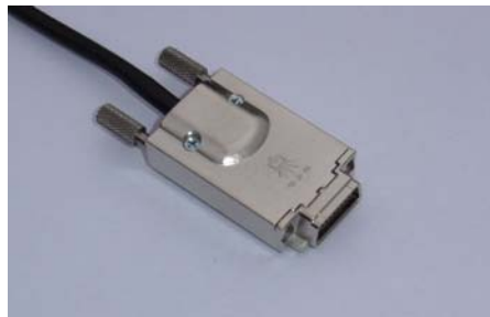
Figure 3 Infiniband type of connector used to connect to a SAS HBA external port (SFF8470)
