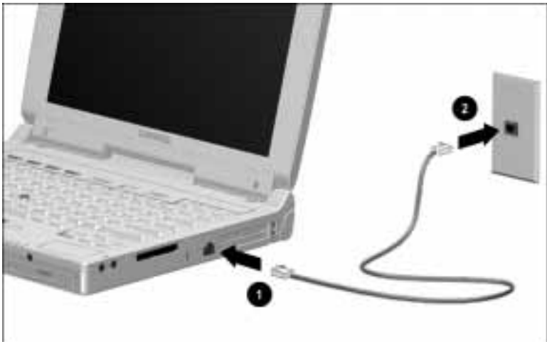
Connecting the Modem to a Telephone Wall Jack in North America, Latin America, Japan, or Hong Kong
