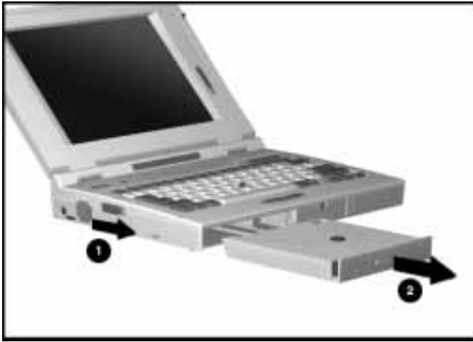
Removing the CD-ROM Drive from the Computer MultiBay
