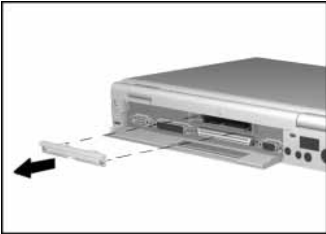
Removing the Memory Slot Cover
