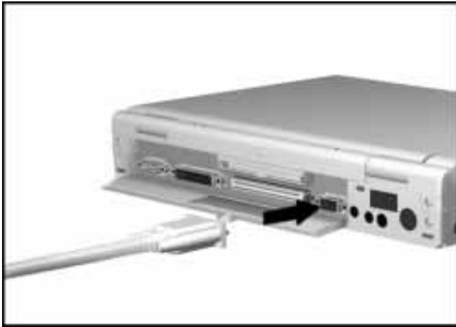
Connecting an External Monitor to the Computer
