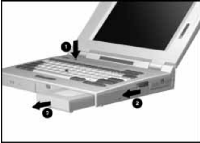
Removing a Battery Pack from the Computer
