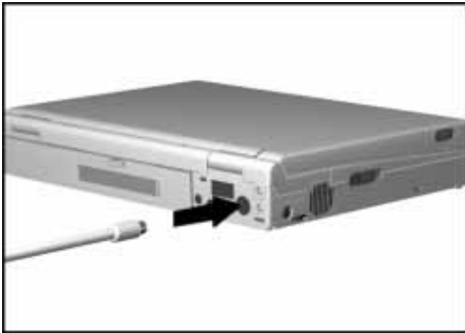
Connecting an External Keyboard, Keypad, or Pointing Device
