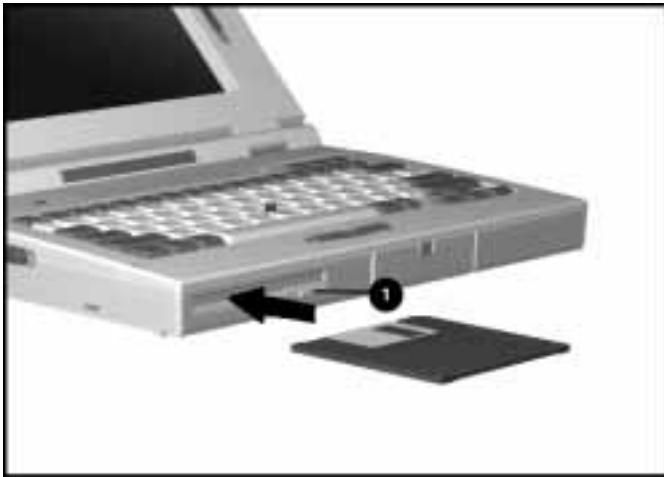
Inserting a Diskette into the Diskette Drive
