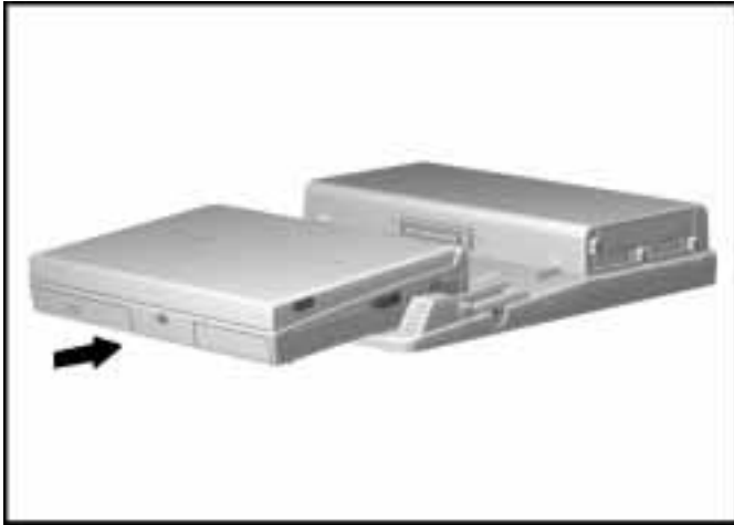
Sliding the Computer into the Expansion Base
