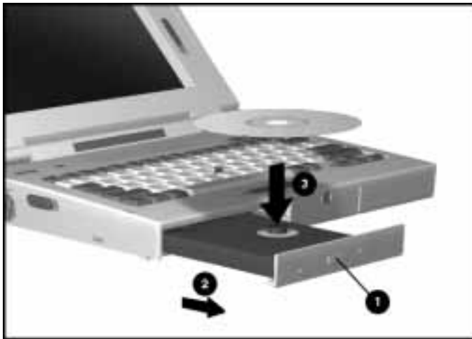
Placing a CD into the CD Loading Tray
