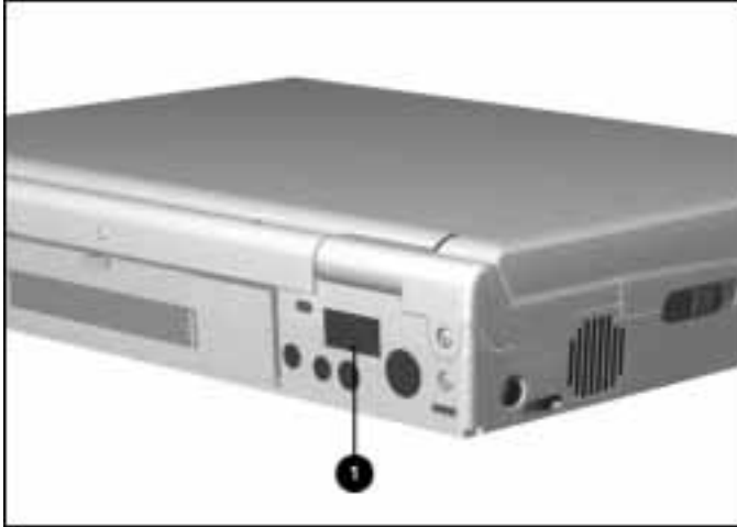
Infrared Port on the Computer
