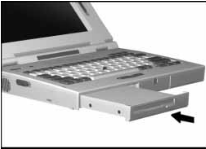
Inserting the Diskette Drive into the Computer MultiBay
