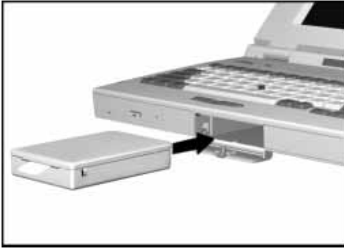
Inserting the Hard Drive into the Hard Drive Bay
