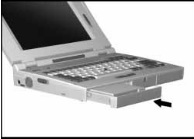
Inserting the MultiBay Hard Drive Carrier into the Computer MultiBay
