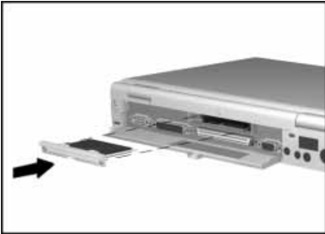
Inserting a Memory Expansion Board into the Memory Slot
