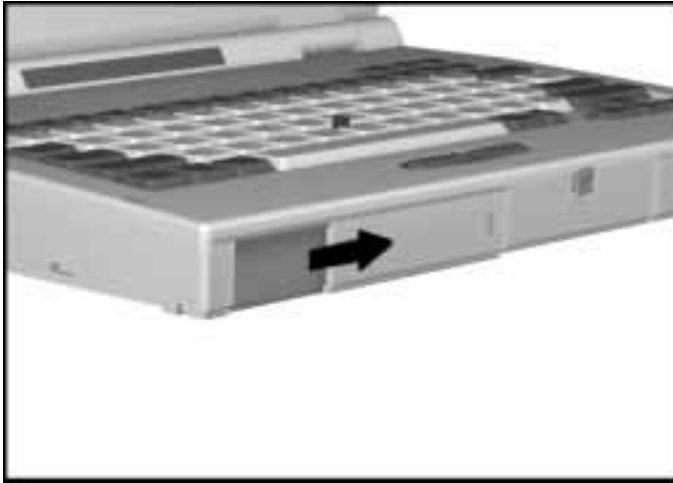
Sliding the Battery Panel to Cover the MultiBay Opening
