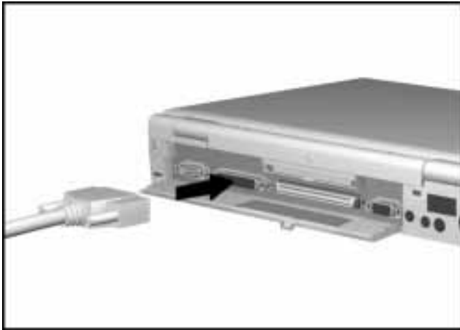
Connecting a Parallel Device to the Computer
