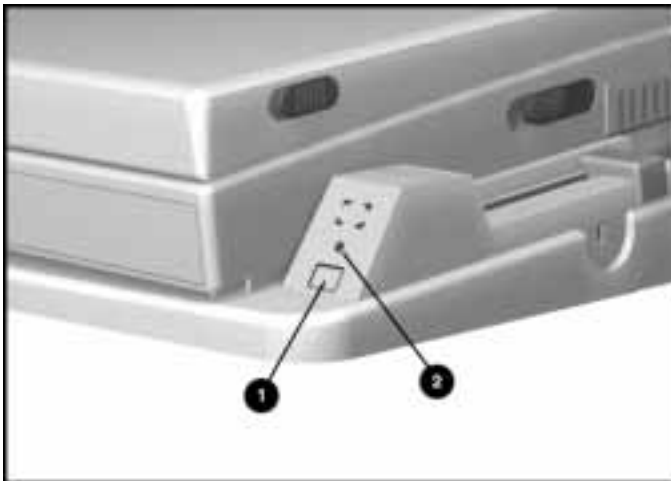
Turning the System On with the Expansion Base Power Button
