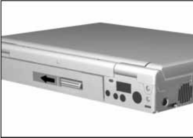
Sliding Open the External Options Connector Cover
