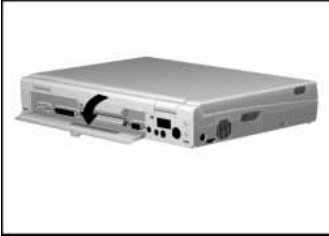
Opening the Connector Door on the Rear Panel
