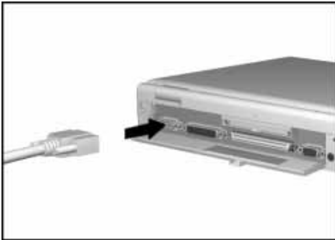
Connecting a Serial Device to the Computer
