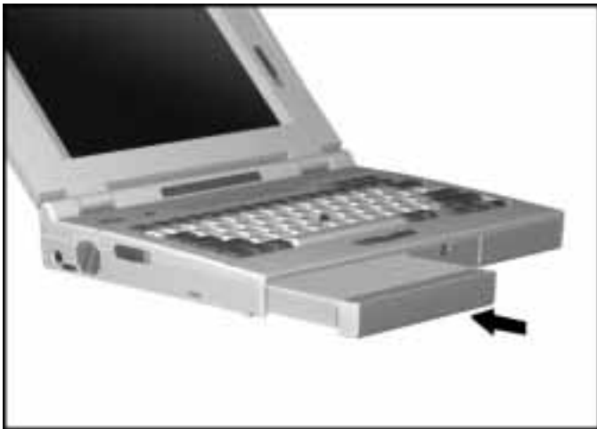
Inserting the MultiBay Weight Saver
