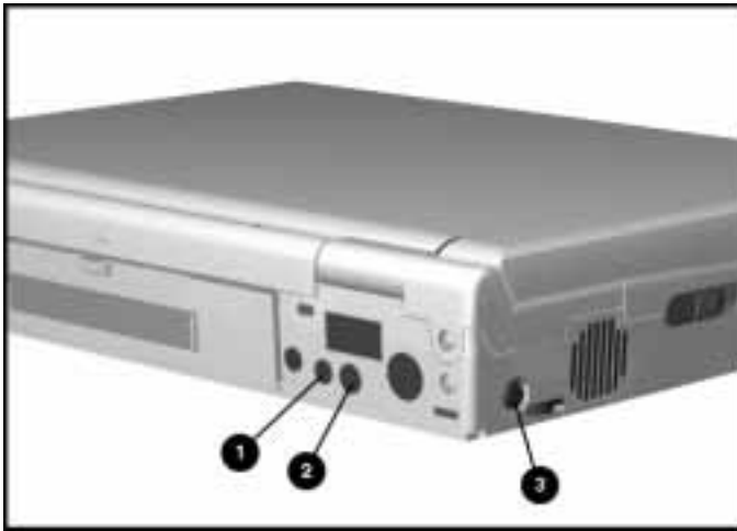
Jacks for Connecting External Audio Equipment
