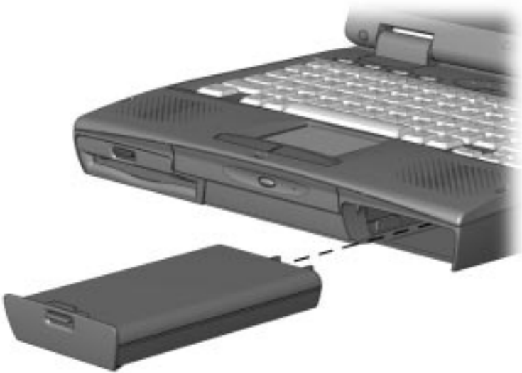
Inserting the Battery Pack into the Battery Bay
