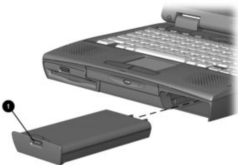
Removing the Battery Pack from the Battery Bay
