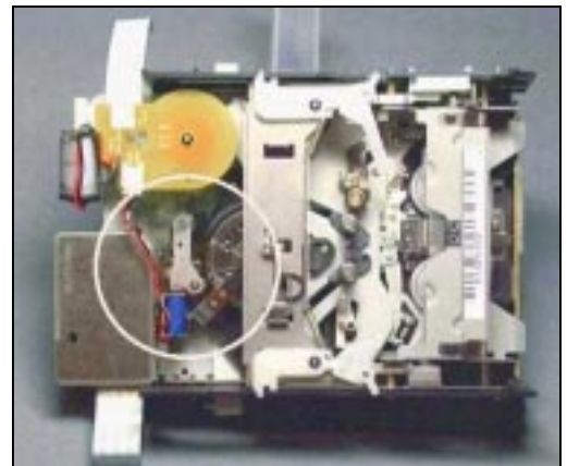
Figure 8: DDS-3 head cleaner in DAT drive.
