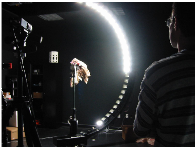
Figure 1: The Light Stage illuminates an artifact (center) from a dense array of incident illumination directions as its appearance is recorded by high-speed digital video cameras (one can be seen in the upper left). This quarter-second photographic exposure shows several of the lights on at once although only one strobe light flashes at any given time.
