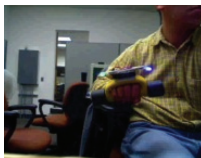
Figure 1. An optical tracking device that utilizes one or two low-cost webcams to track one, two or three diodes providing information of three, five, or six degrees of freedom, developed by Yeh et al. (2008).
