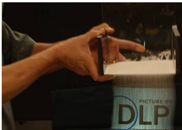
Figure 9 A cascade of retroreflective beads illuminated by a projector. Such a cascade could be used to create virtual elements anywhere within a space.
