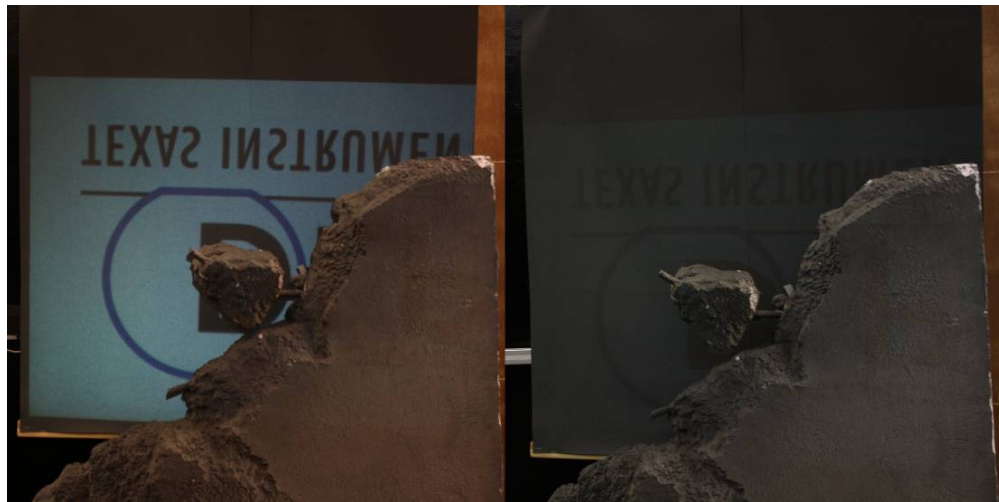
Figure 3 The retroreflected illumination level near the optical axis of the pico-projector (left) is much less than the retroreflected illumination level at 16 inches from the optical axis (right). This screen was placed behind a concrete wall prop.
