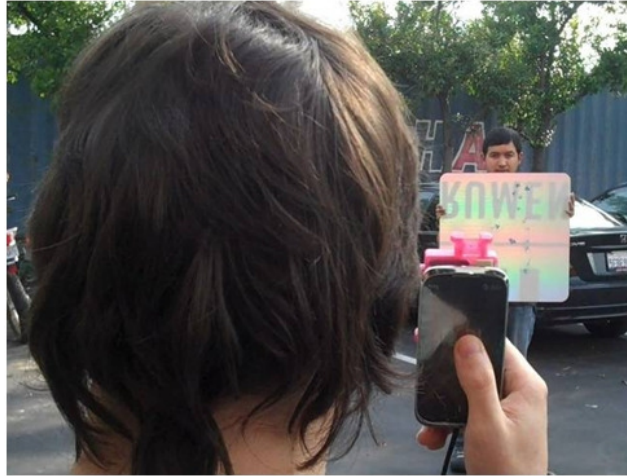
Figure 4 A test of retroreflective sign material and a projector/mobile phone during daylight. The projection is still very discernable to the user.
