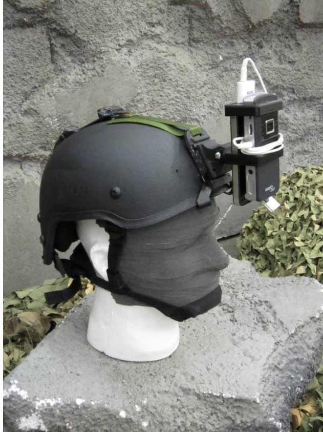
Figure 6 A prototype REFLCT module, powered by a smartphone, is compact enough to attach to a night vision goggle mount for military training.
