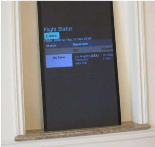
Fig. 12 A “cheek-based” cell phone display could present personalized information, like flight status, on a public retroreflective surface
