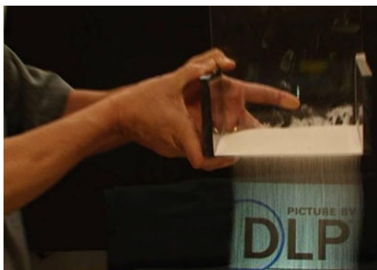
Fig. 9 A cascade of retroreflective beads illuminated by a projector. Such a cascade could be used to create virtual elements anywhere within a space
