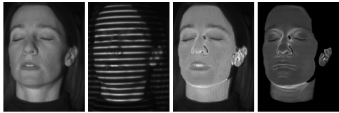
Figure 1: (a) Face lit by the fully on projector, (b) one of 40 phase-shifted stripe patterns, (c) after correcting for lambertian light attenuation, (d) estimate of indirect light from subtracting the minimum of each pixel’s profile.
