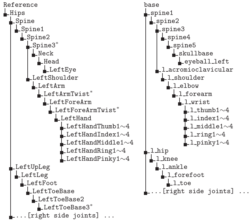
Figure 3. Final mapping result achieved by our system—left side is given as an example following MOTIONBUILDER naming convention, and right side is the corresponding joint names in our system. * denotes joint (if exists) is skipped as it is not handled by our system.
