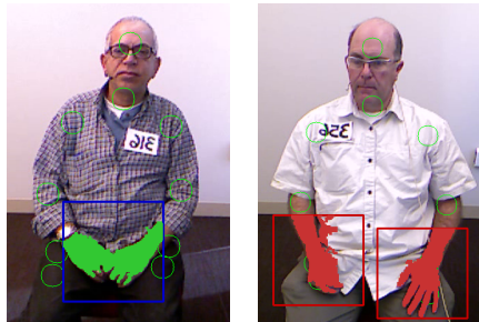
Figure 1: Example results of our hand segmentation approach. Green circles represent the original skeleton tracking data, and the rectangles indicate the search area within the depth and color images.
