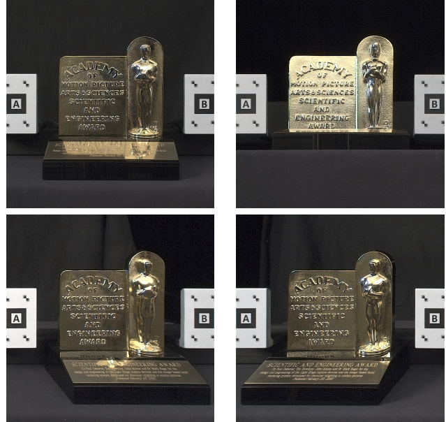
Figure 3. 640 \times 640 pixel undistorted, rectified, and sharpened images with the outer fiducials stabilized and chromatic aberration removed.
