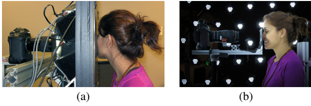
Figure 2: Acquisition setups for skin microgeometry (a) Twelve-light hemispherical dome (at end of camera lens) capturing a cheek patch. (b) LED Sphere capturing the tip of the nose, with the camera inside the sphere.
