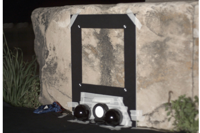
Figure 3: BRDF Samples are measured from a 30cm square region exhibiting a representative set of surface reflectance properties. The technique used a hand-held light source and camera and a calibration frame to acquire the BRDF data quickly.
