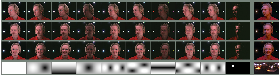
Fig. 2: An actor stands within a sphere of inward-pointing LED lights as elements of the spherical harmonic lighting basis (bottom) are projected in rapid succession during each extended frame. Linear combinations of the frames produce novel illumination on the performance according to a sampled lighting environment (right).
