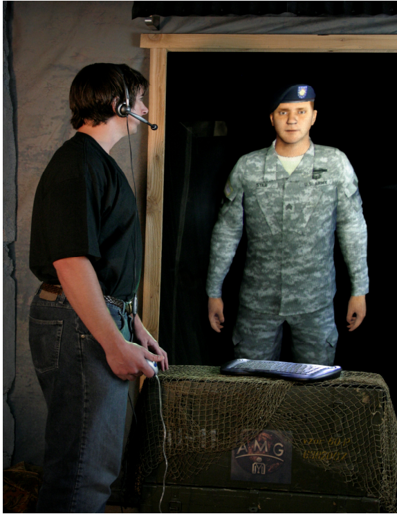
Figure 3: A virtual human character who uses spoken dialogue to understand and answer questions about military careers.
