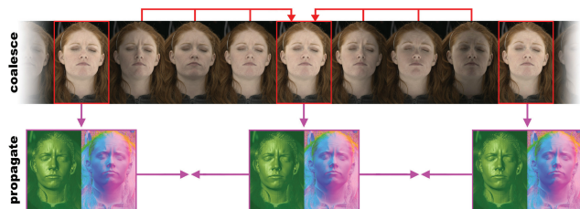
Fig. 3. An illustration of joint alignment and upsampling: Photometric normals are computed at tracking frames after joint alignment of gradient illumination conditions and their complements (red arrows). Base geometry is computed at the tracking frames from dense stereo correspondences. Both photometric normals and base geometries are then warped and blended at target intermediate frames (magenta arrows).
