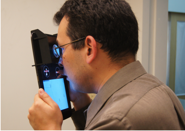
Figure 1: The iNVerse immersive viewer transforms a tablet device into a stereoscopic 3D display with integrated inertial tracking and a multi-touch surface for interaction and control.
