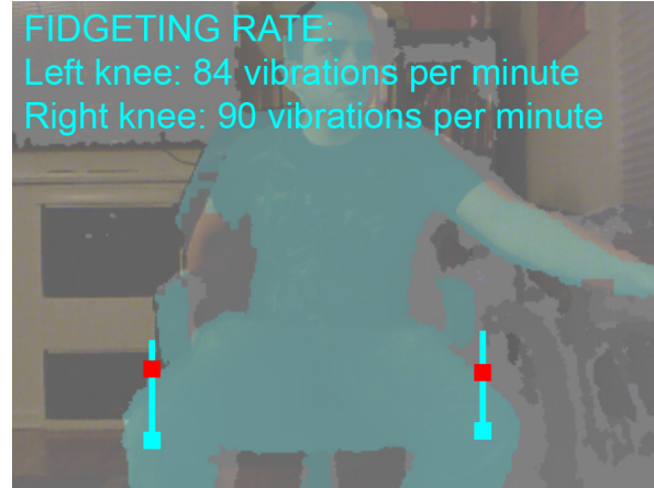
Figure 2. Measuring “leg jiggling” fidgeting behavior with the Microsoft Kinect sensor. The two vertical lines show the approximate knee position returned from the skeleton tracker (cyan dot) as well as the point along the surface of the leg that is used to measure leg oscillation (red dot).
