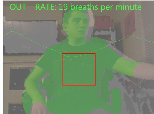
Figure 1. Measuring breathing with the Microsoft Kinect sensor. The graphed line shows the cyclical fluctuation of the chest cavity expansion and contraction from inhalation and exhalation. The breathing state (IN or OUT) along with the respiratory rate is also displayed on screen.
