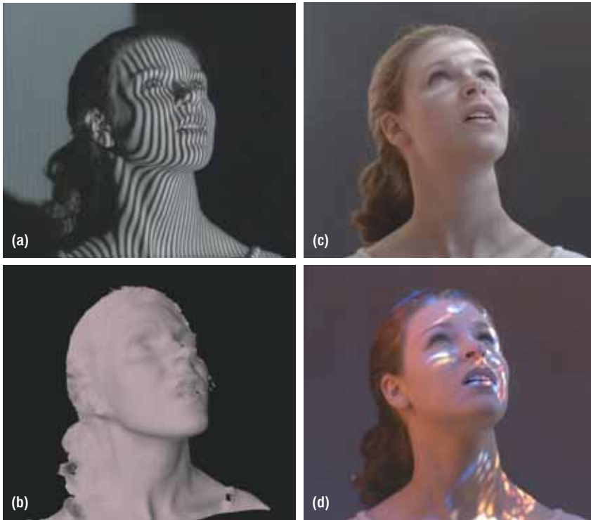
Figure 5. Simulating spatially varying illumination on an actor's performance. (a) The actor is lit by a structured illumination pattern from a high-speed video projector. (b) A geometric model is derived for a frame of the performance. (c) The actor is virtually illuminated as if in a room with sunlight streaming through Venetian blinds. (d) The actor is virtually illuminated as if in a cathedral with light projected from a stained glass window.
