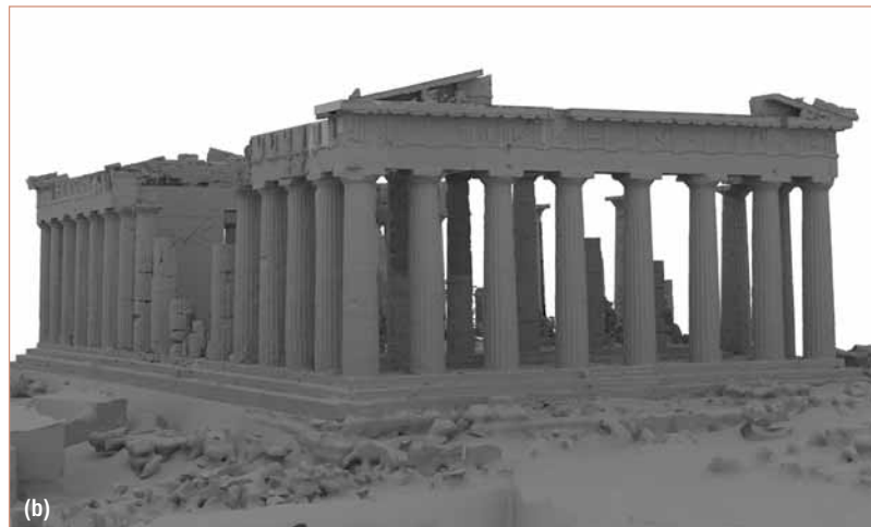
Figure 7. Capturing the lighting and geometry of the Parthenon. (a) A light probe device records incident lighting conditions near the base of the temple. (b) A 3D surface model of the scene geometry obtained using 3D laser scanning.
