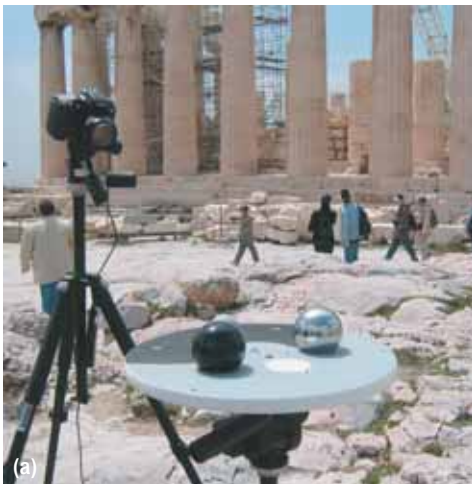
Figure 7. Capturing the lighting and geometry of the Parthenon. (a) A light probe device records incident lighting conditions near the base of the temple. (b) A 3D surface model of the scene geometry obtained using 3D laser scanning.
