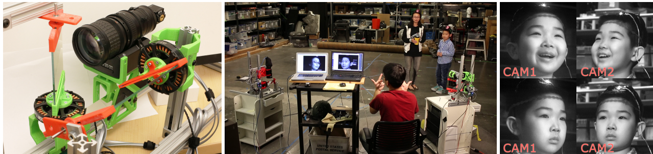
Figure 1: (Left) A stationary camera with an instrumented zoom & focus lens attached to motorized pan/tilt mirrors. (Middle) Two units of our virtual head-mount camera setup in a performance capture stage for facial tracking. (Right) Frames from a tracked facial performance.
