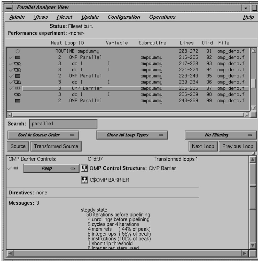
Figure 28. Loops Using C\$OMP BARRIER Synchronization
