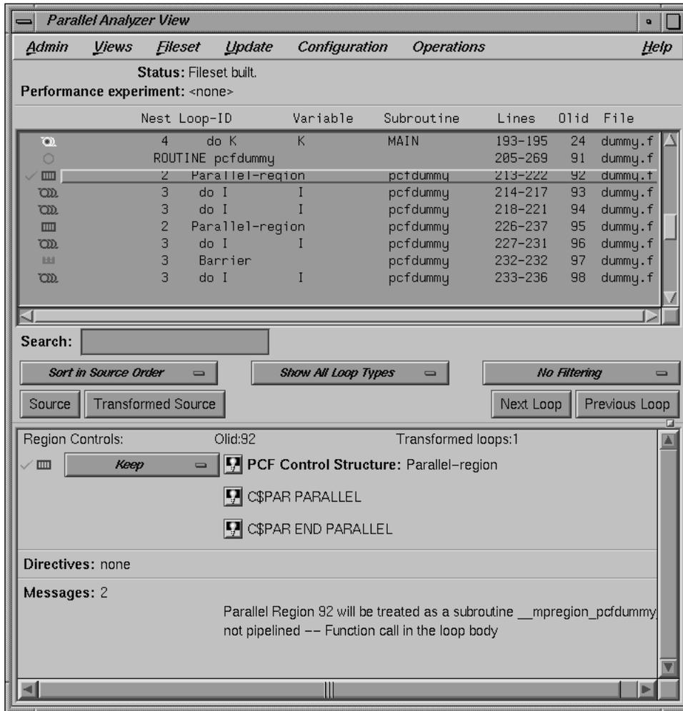
Figure 79. Explicitly Parallelized Loops Using C\$PAR PDO
