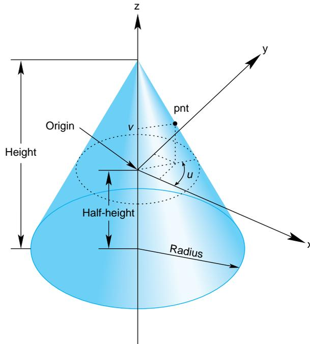
Figure 11-14 Cone Parameterization
