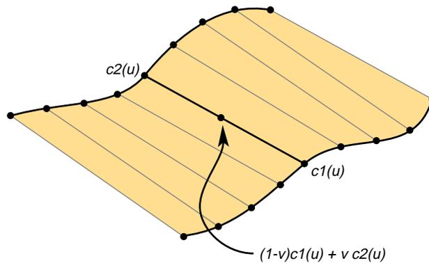
**Figure 11-16** Ruled Surface Parameterization
