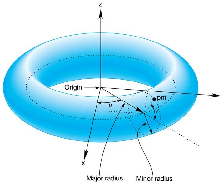
Figure 11-13 Torus Parameterization
