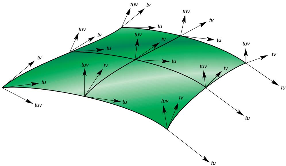
**Figure 11-19** Hermite Spline Surface With Derivatives Specified at Knot Points
