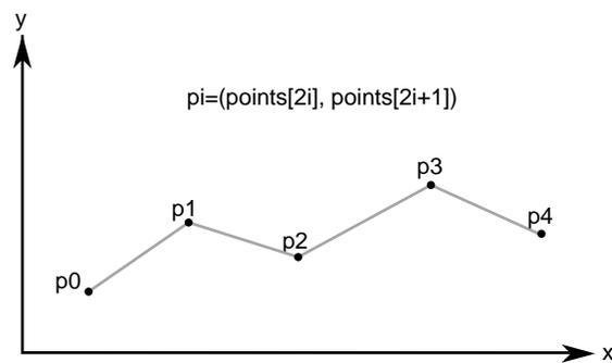
Figure 11-7 Discrete Curve Definition
