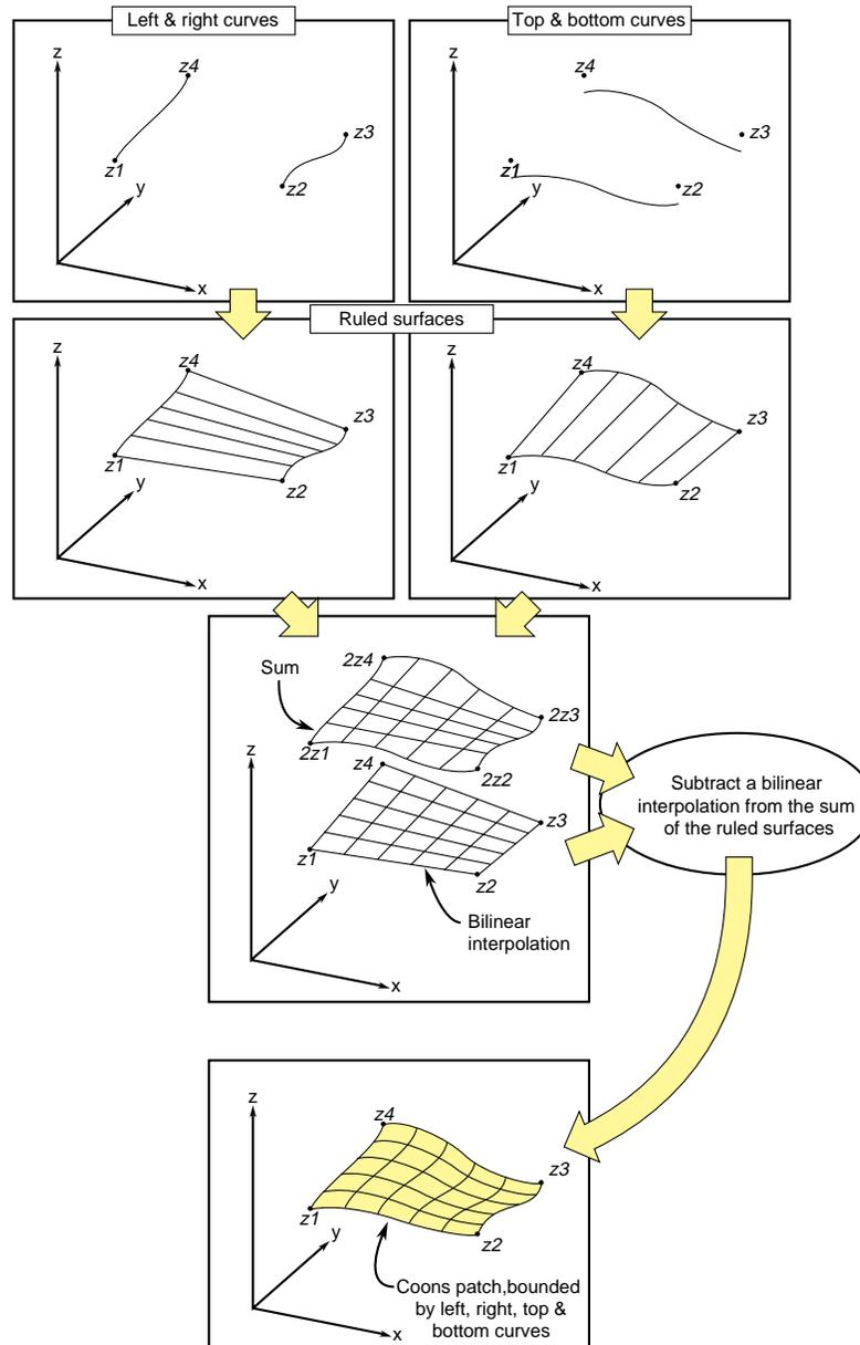
Figure 11-17 Coons Patch Construction
