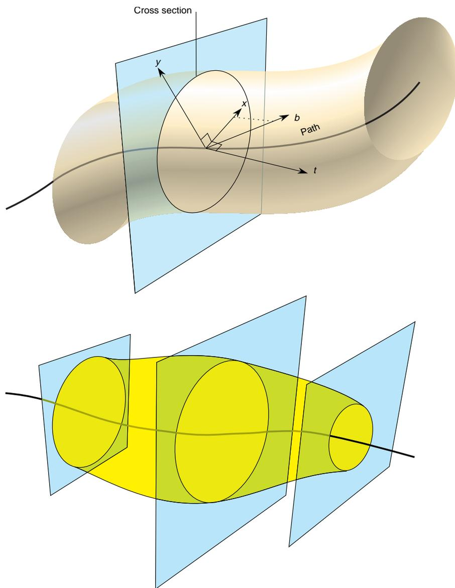
**Figure 11-15** Swept Surface: Moving Reference Frame and Effect of Profile Function
