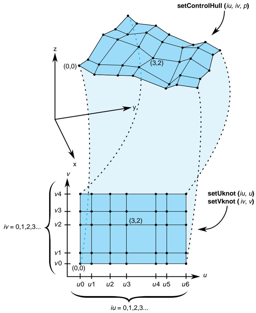
Figure 11-18 Nurb Surface Control Hull Parameterization
