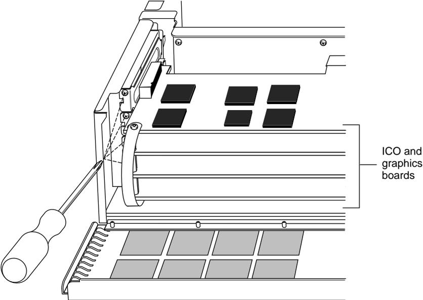
**Figure 1-26** Attaching the Graphics Board Set to the Chassis
