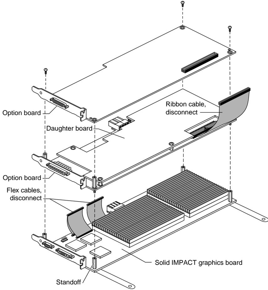
**Figure A-2** Solid IMPACT Graphics Board With Option Boards
