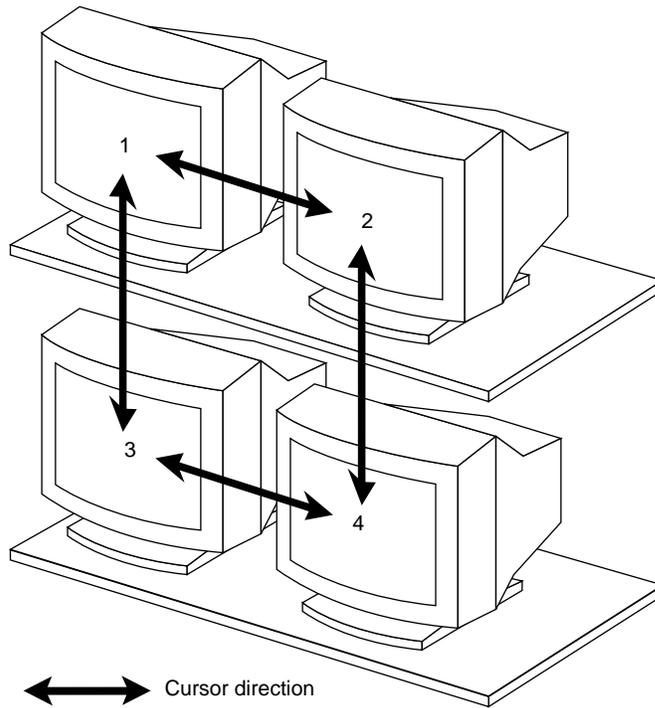
**Figure 2-4** Moving the Cursor Between Monitors
