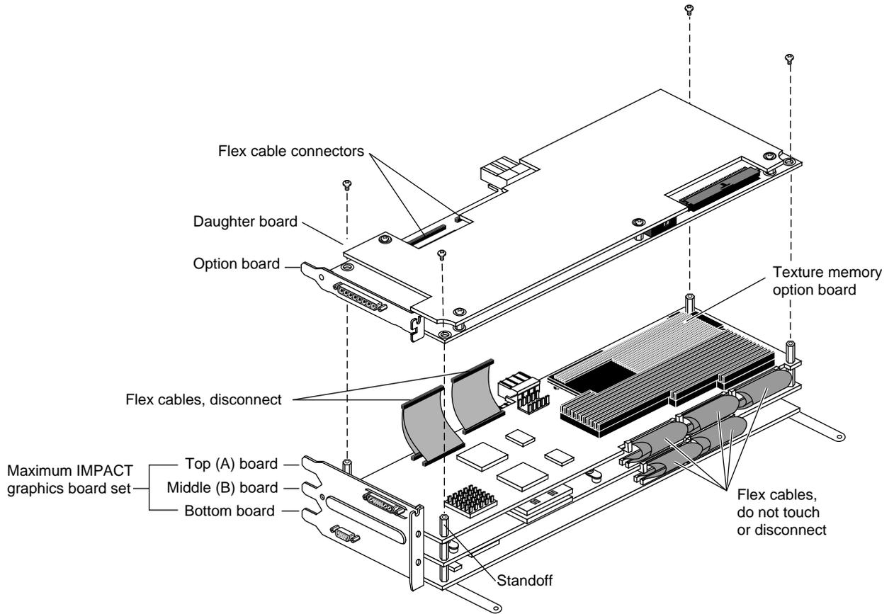
**Figure A-4** Maximum IMPACT Graphics Board Set With Option Boards
