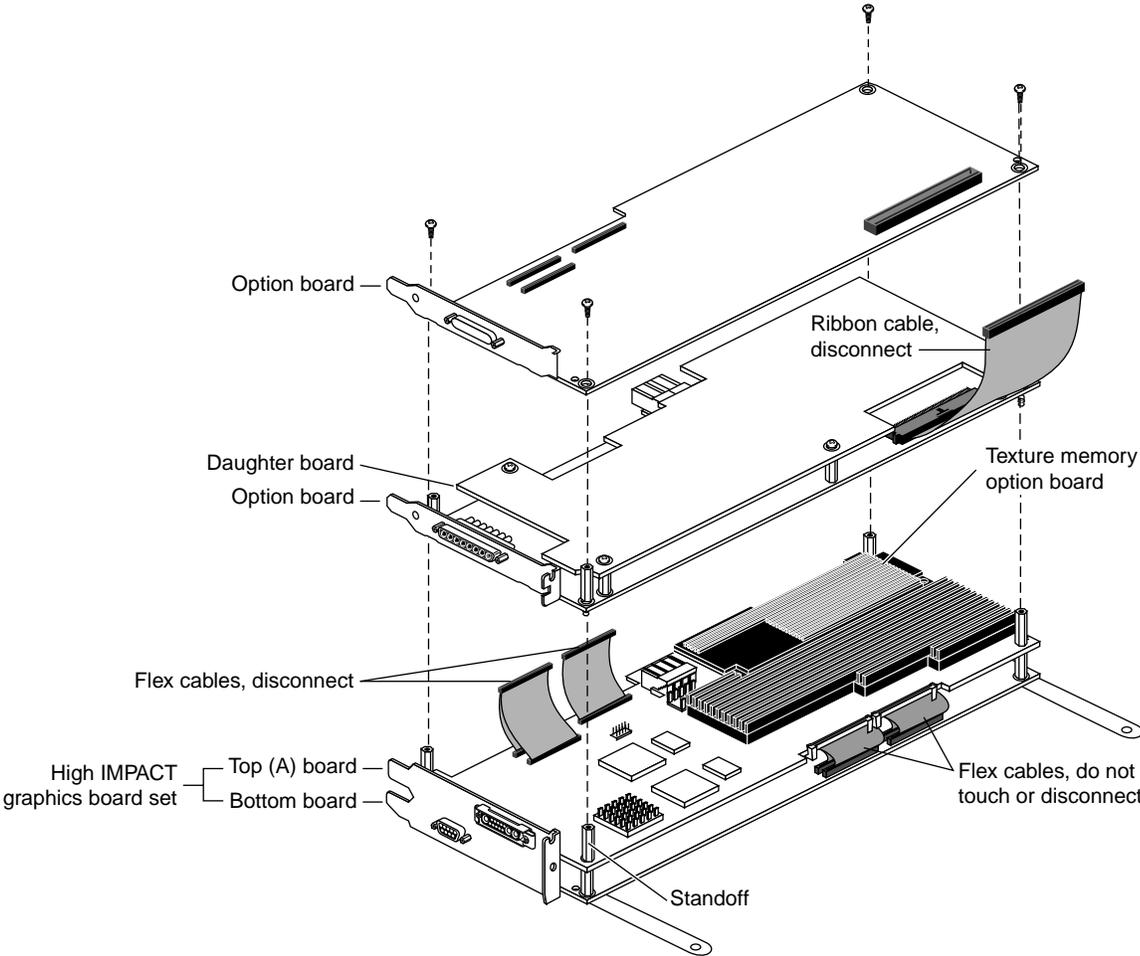
Figure A-3 High IMPACT Graphics Board Set With Option Boards
