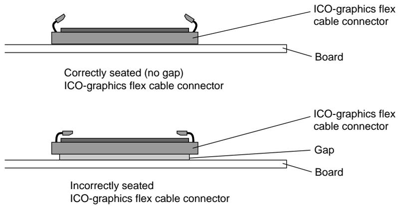
**Figure 1-18** Seating the ICO-Graphics Flex Connectors
