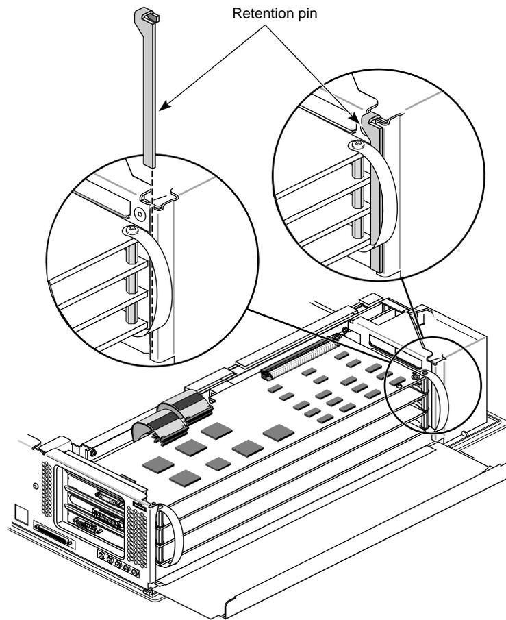
**Figure 1-27** Replacing the Retention Pin
