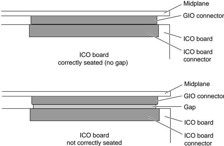
**Figure 1-25** Checking the Seating of the GIO Connector
