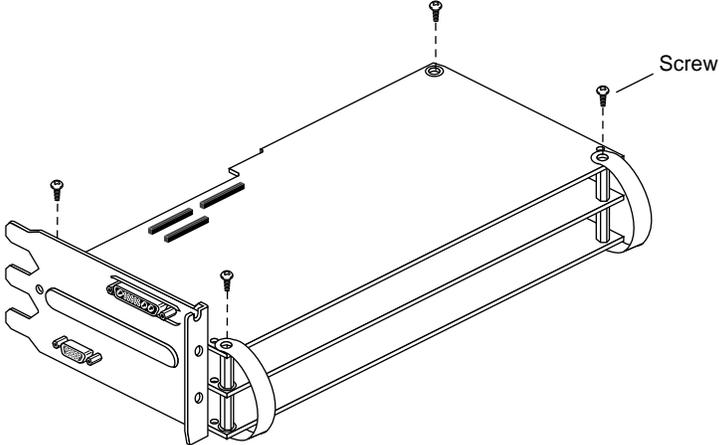
**Figure 1-11** Removing Graphics Board Set Screws
