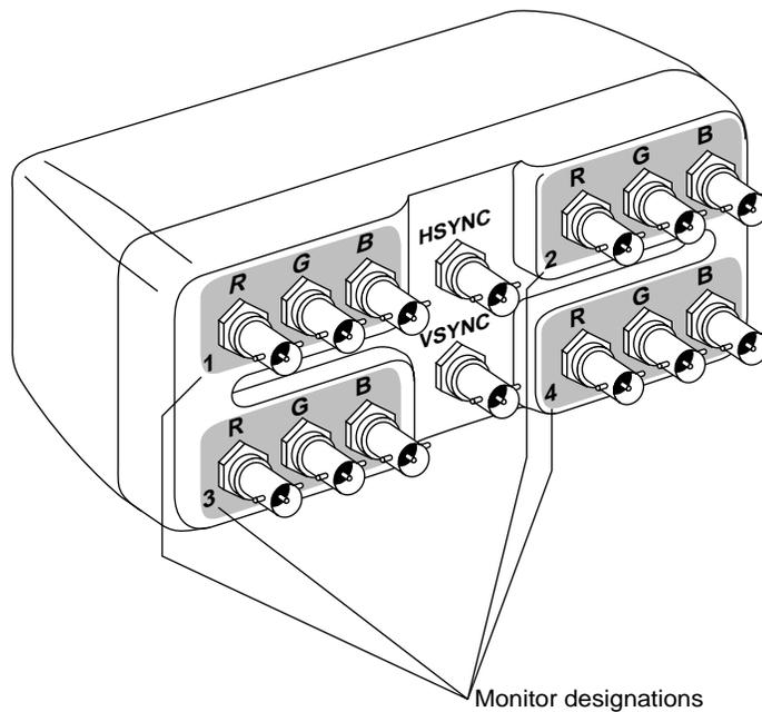
**Figure 2-2** Connecting the Breakout Box to Four Monitors
