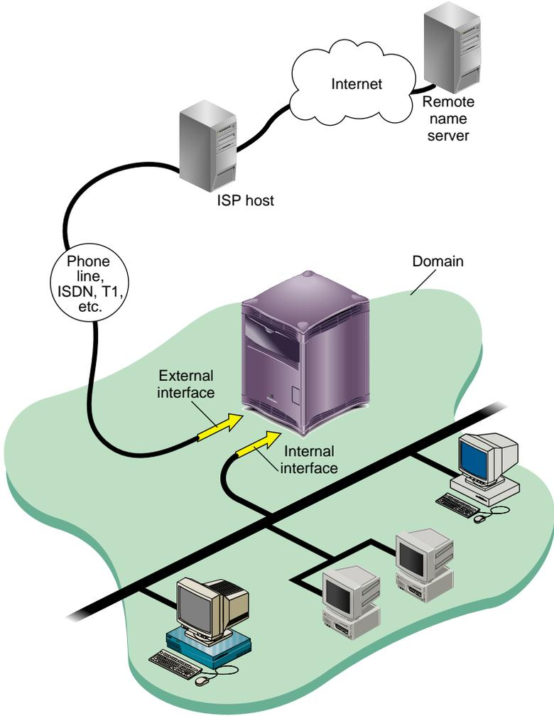
Figure 1-1 WebFORCE Internet Gateway Connection to the Internet
