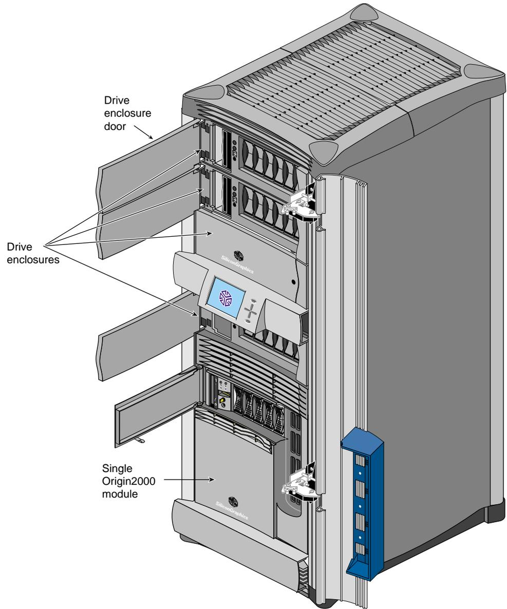
**Figure 4-3** Single Origin2000 Module in a Rack with Four Origin Vault Drive Boxes
