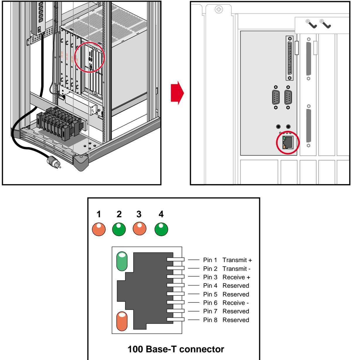
Figure 3-1 Standard Ethernet on Origin2000 Rackmount
