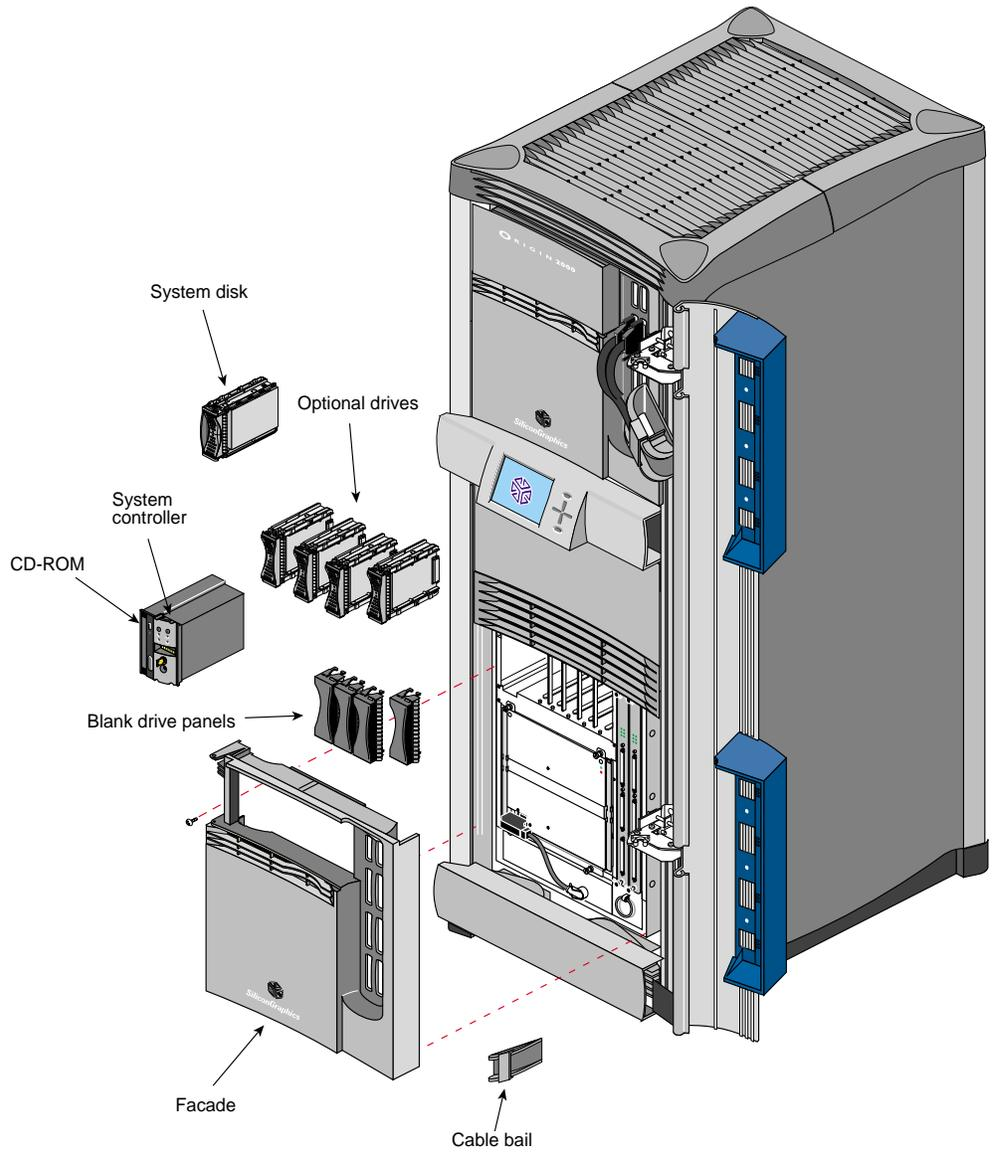
**Figure 6-1** Customer-Replaceable Units (CRUs) for the Origin2000 Rackmount System
