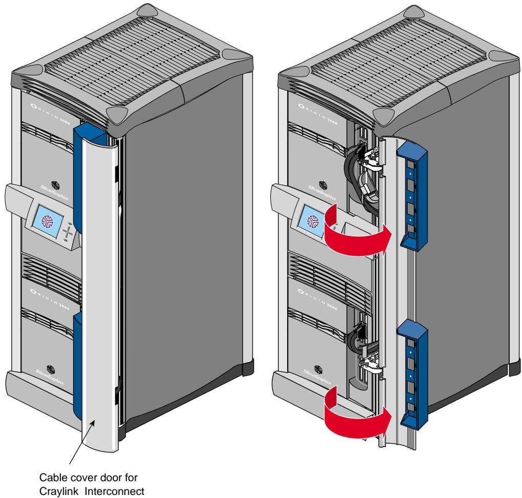
**Figure 6-8** Opening the Cable Cover Door
