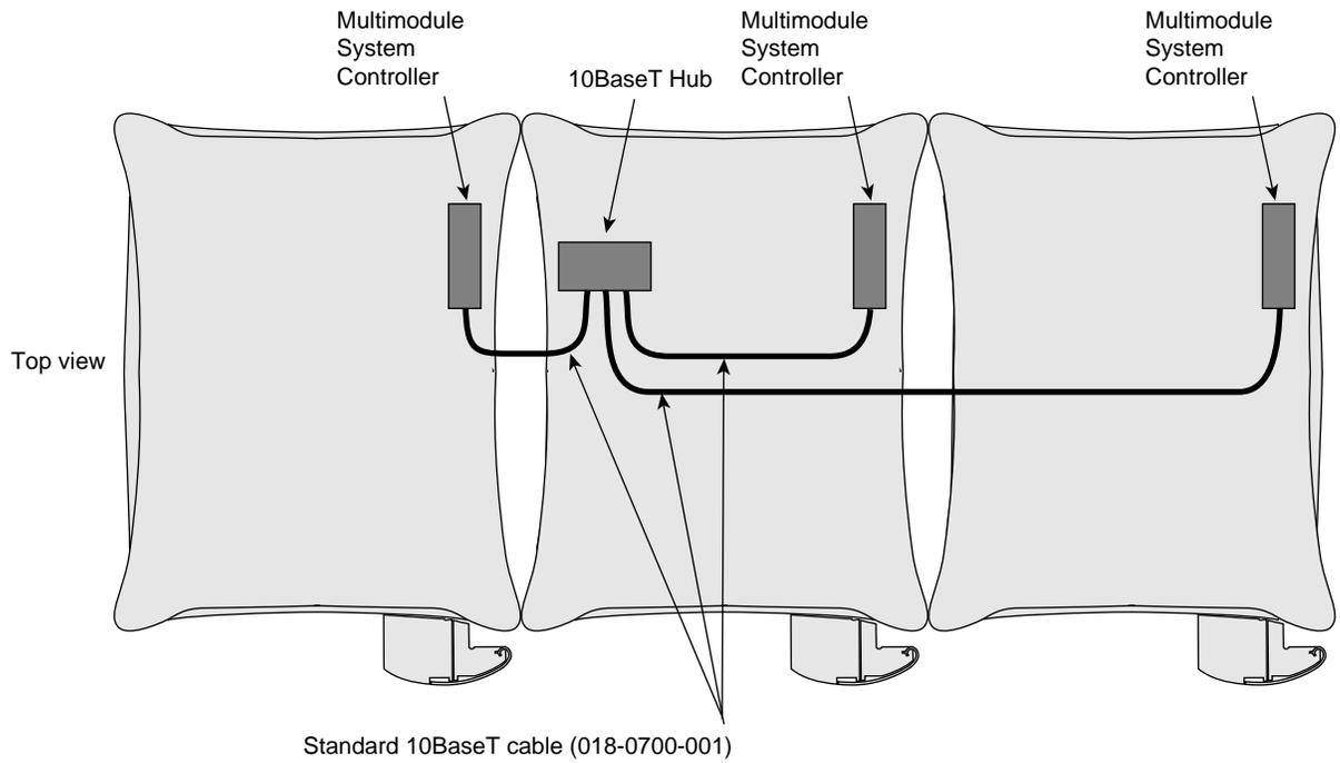
**Figure 7-7** MMSC to 10BaseT-Hub 1BaseT Ethernet Cabling (2 racks)
