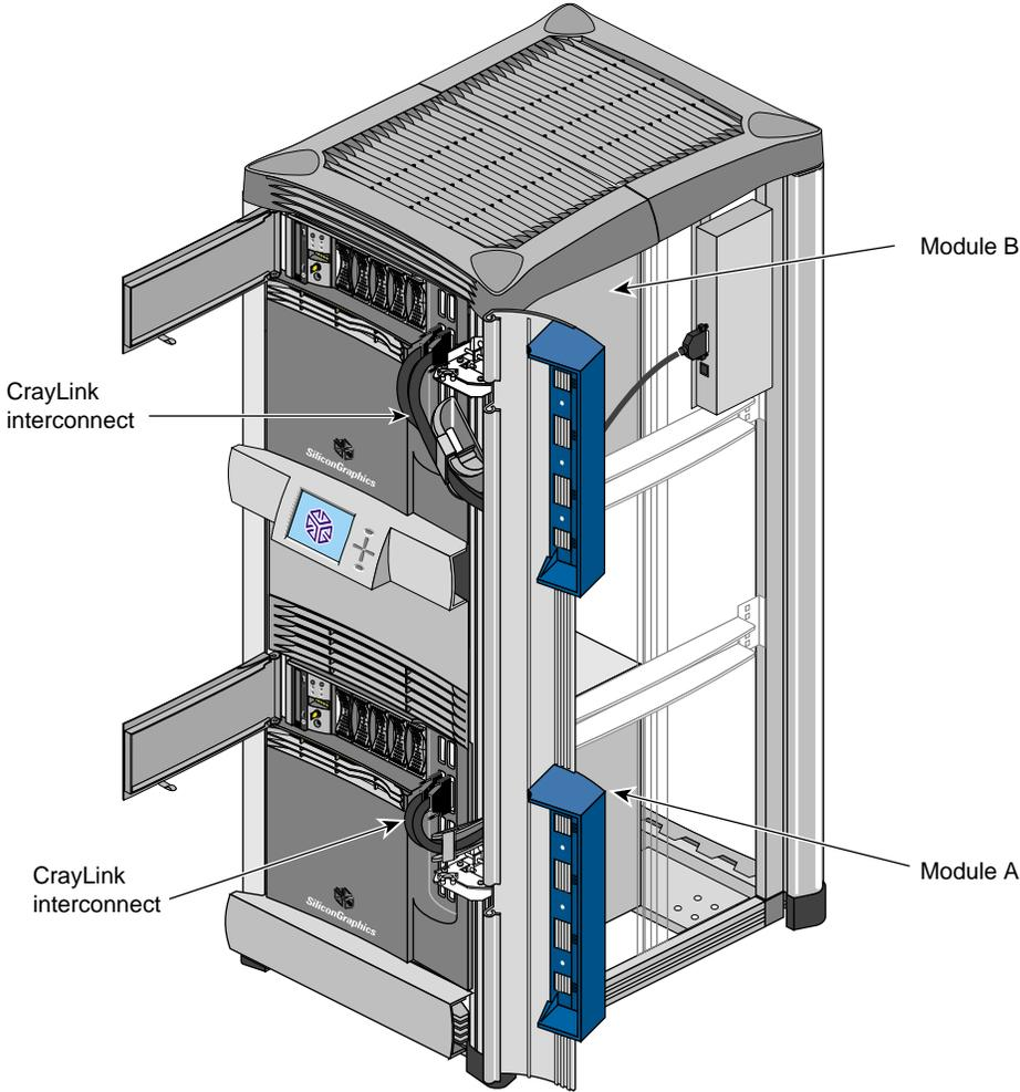
**Figure 1-4** Origin2000 Rackmount Chassis (Side Panel Removed)
