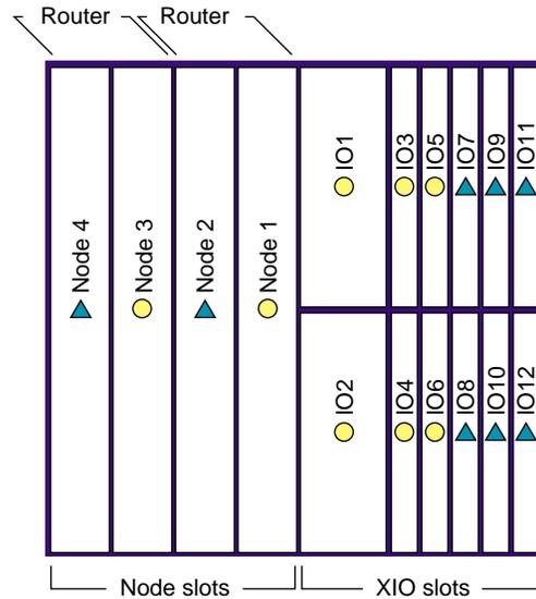
**Figure 2-3** Board Configuration and Layout for System Module
