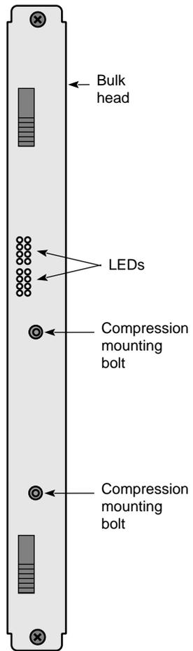
**Figure 2-8** Front View of Node Board Showing Bulkhead
