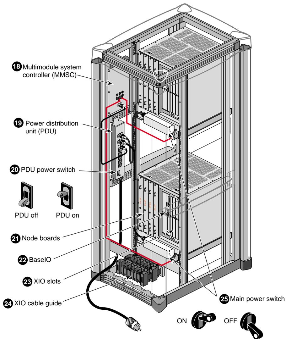
**Figure 2-2** Origin2000 Rackmount Rear View
