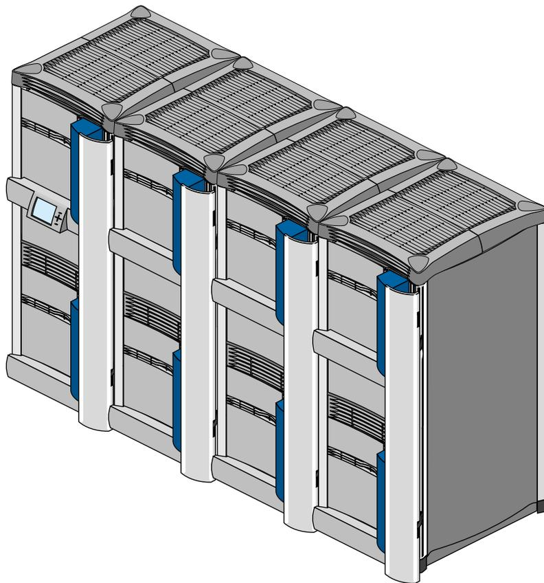
**Figure 1-3** Origin2000 Multitrack Configuration (Four Racks Shown)
