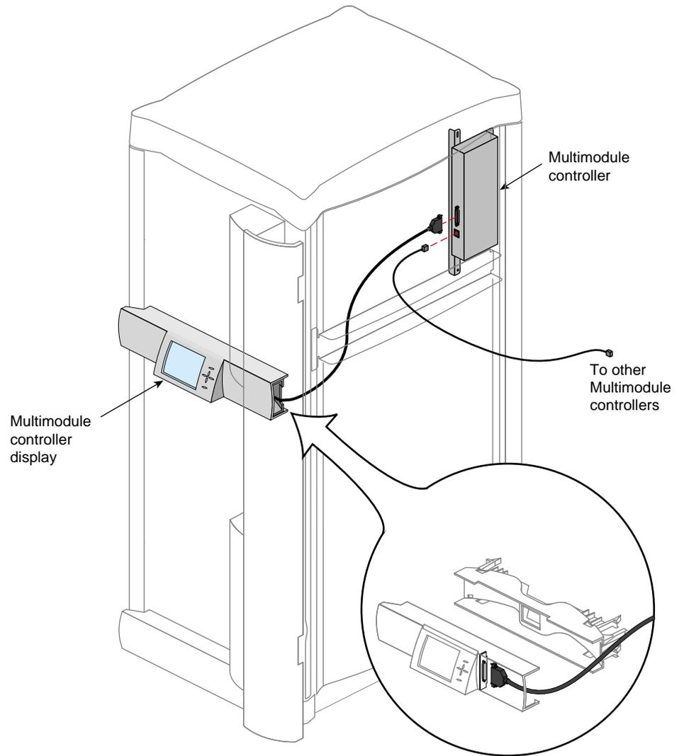
**Figure 7-2** The MMSC and Front Panel
