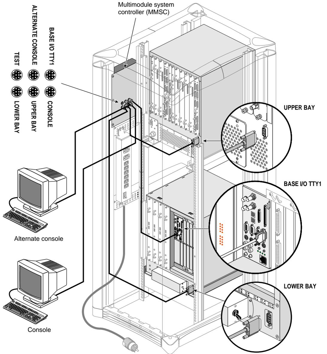
Figure 7-5 MMSC Cabling
