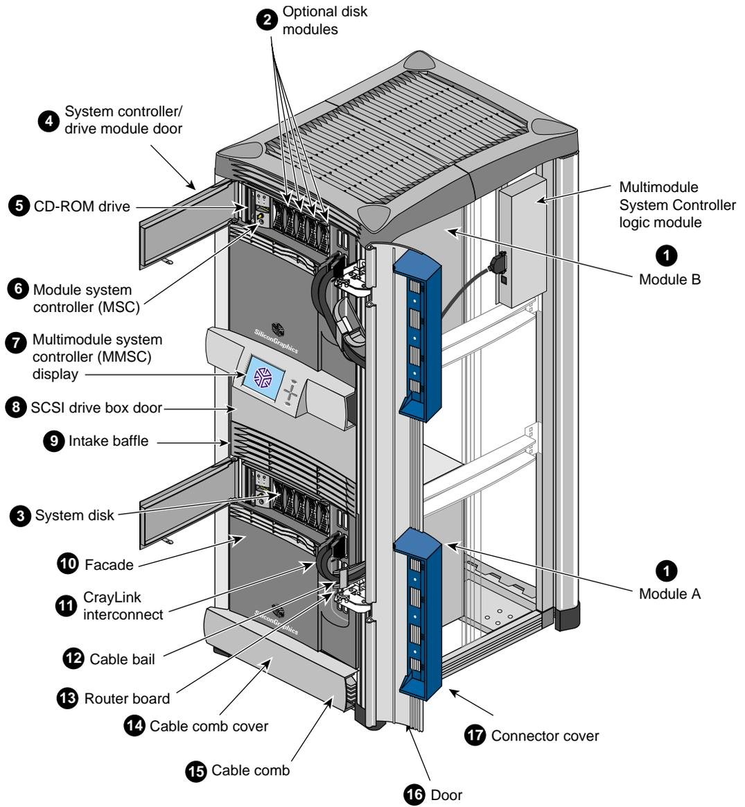
**Figure 2-1** Origin2000 Rackmount System (Front View)
