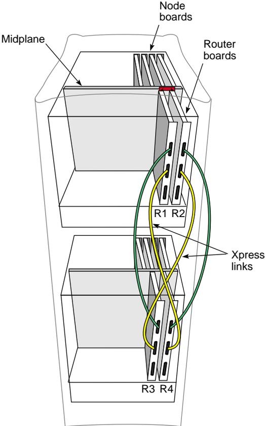
**Figure 4-5** 16P Origin2000 Rackmount with Xpress Links
