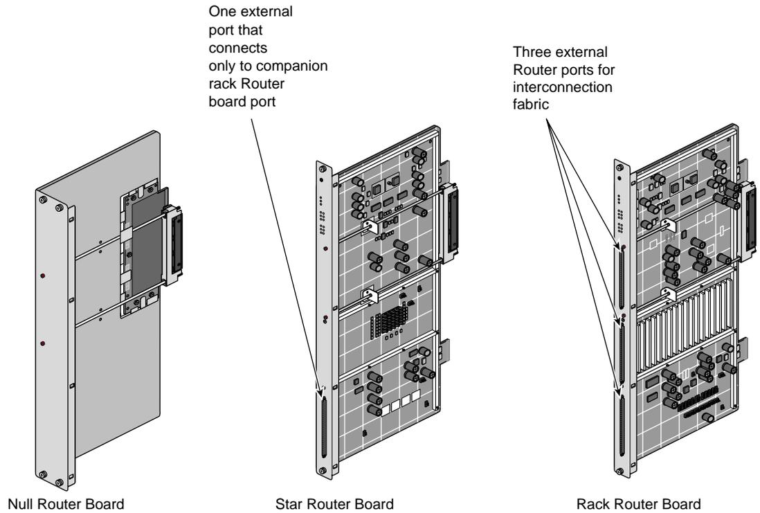
**Figure 2-9** Origin2000 Router Boards
