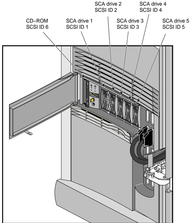
**Figure 5-3** SCSI Hardwire Addresses for the Origin2000 Chassis
