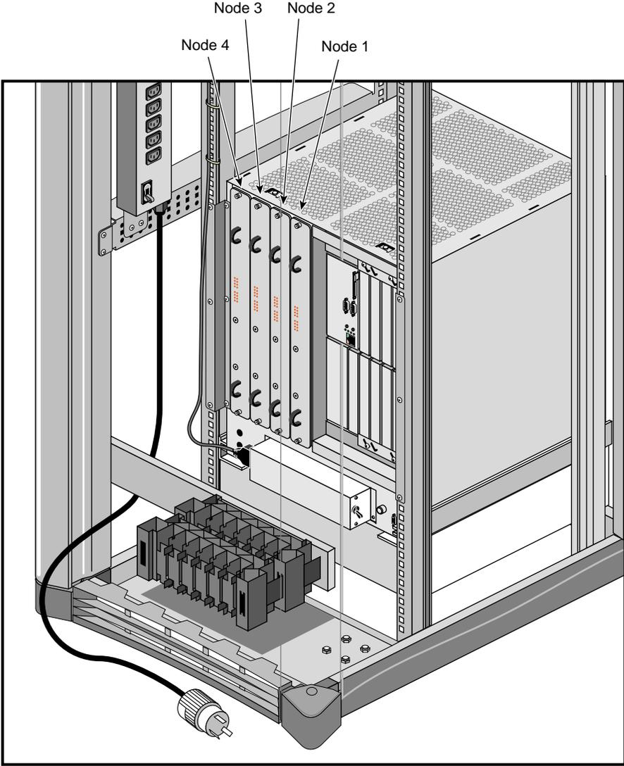
Figure 2-7 Node Board Positioning in the Chassis
