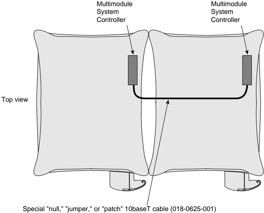
**Figure 7-6** MMSC to MMSC 10BaseT Ethernet Cabling (2 racks)
