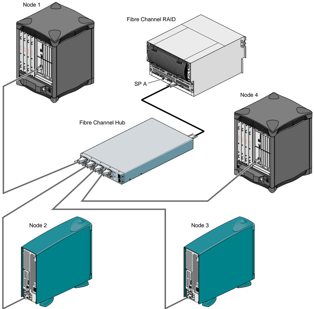
**Figure 2-2** Single-Loop Configuration Example, Fibre Channel RAID Storage
