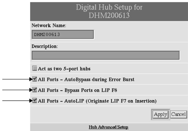
**Figure 5-8** Bypassing Ports
