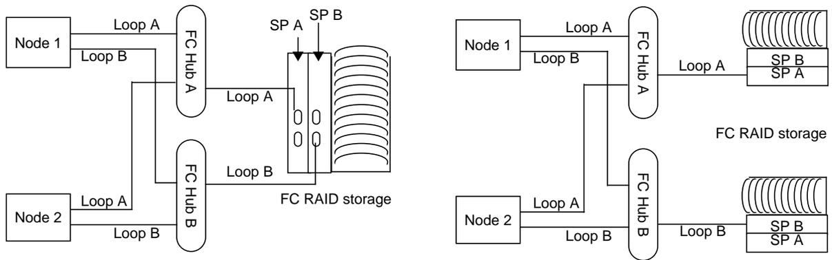
**Figure 2-3** Dual-Loop Configurations With Fibre Channel RAID Storage
