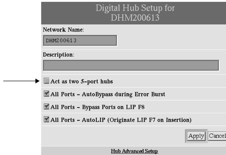
**Figure 4-6** Segmenting and Unsegmenting the Hub
