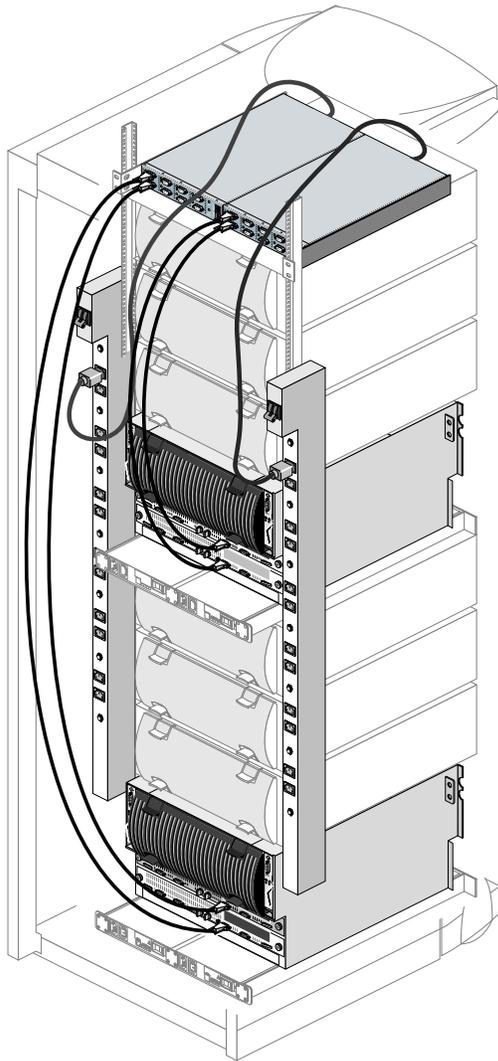
**Figure 1-3** Fibre Channel Rack: Rear View, With Two Fibre Channel Hub Units
