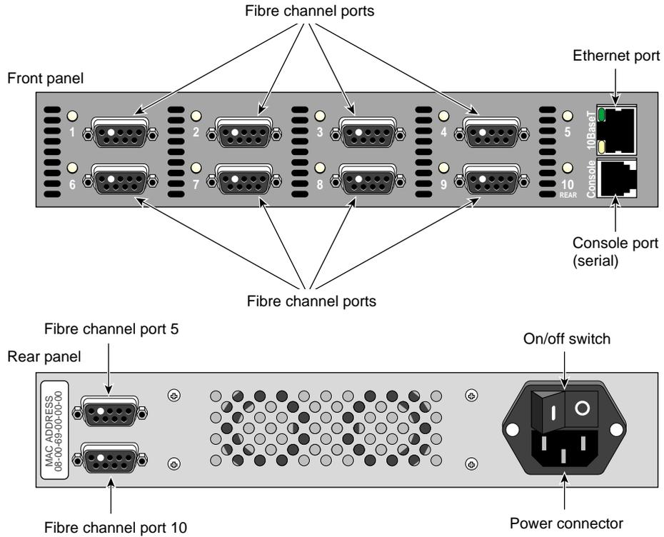
**Figure 1-4** Fibre Channel Hub Ports
