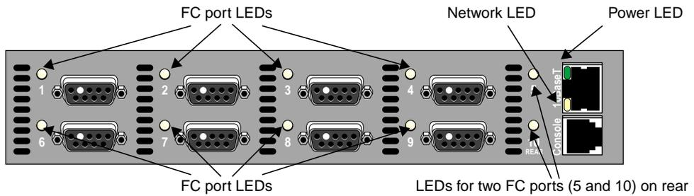
**Figure 3-7** Hub LEDs
