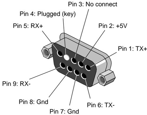
**Figure A-1** Fibre Channel Hub DB-9 Pinout
