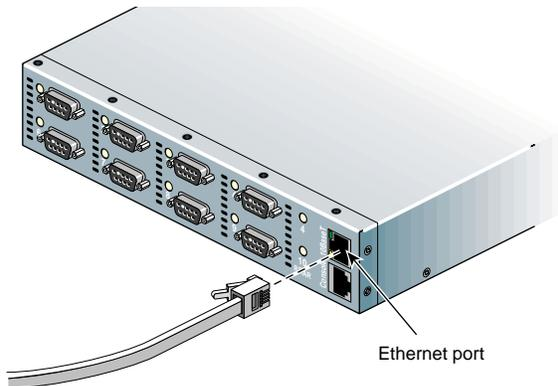
**Figure 3-3** Cabling the Ethernet Port
