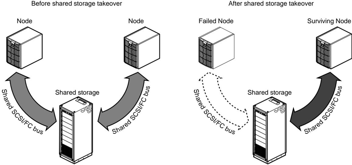
Figure 1-8 Disk Storage Failover in a Two-Node Cluster
