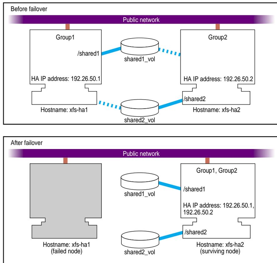
**Figure 2-4** Shared Disk Configuration for Dual-Active Use
