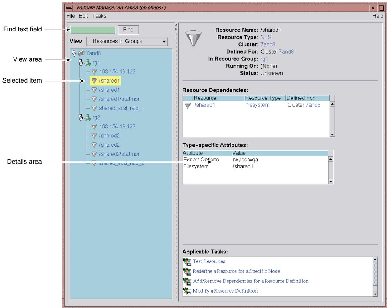
**Figure 5-1** GUI Showing Details for a Resource
