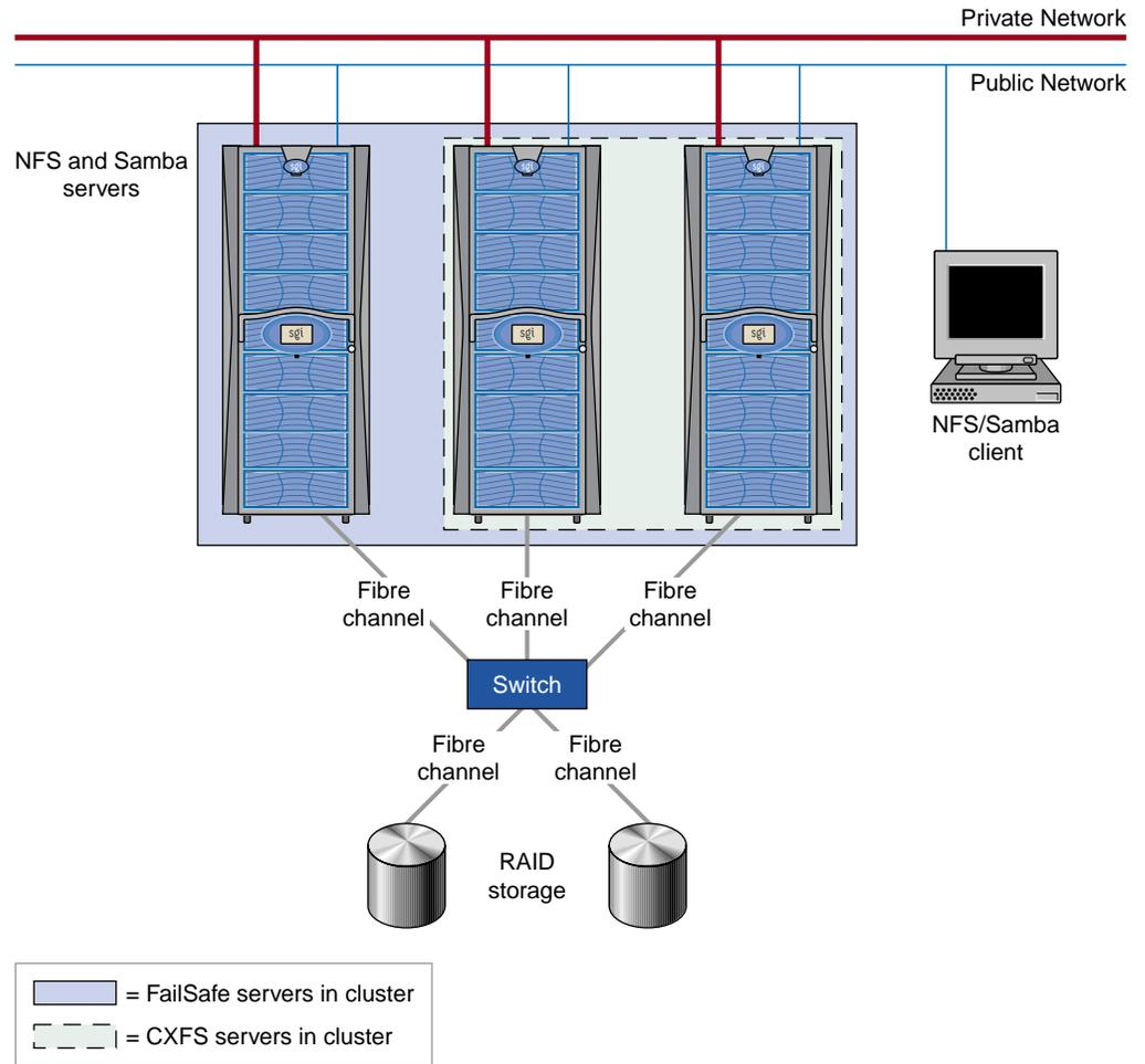
**Figure 1-1** An Example CXFS and FailSafe Configuration
