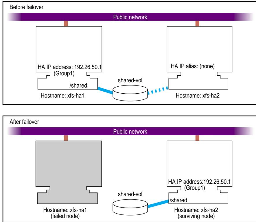
**Figure 2-3** Shared Disk Configuration for Active/Backup Use
