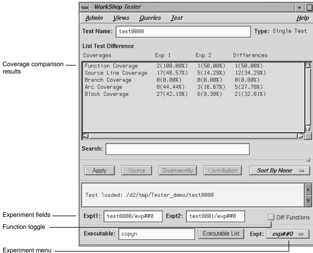
Figure 5-26 Compare Test Example — Coverage Differences
