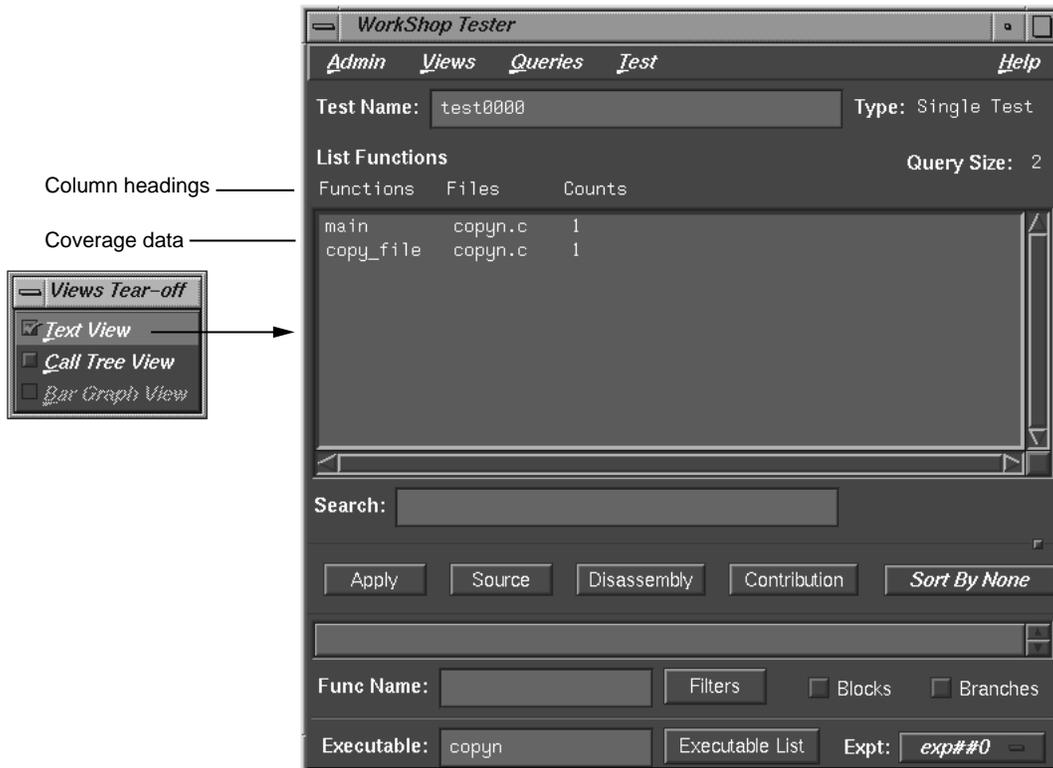
**Figure 5-11** List Functions Query in Text View Format
