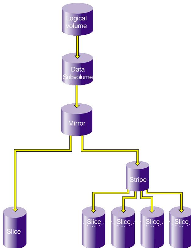
**Figure 5-21** Filesystem after Attaching Stripe to Mirror
