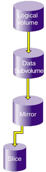
**Figure 5-20** Filesystem after Insertion of Mirror
