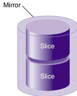
**Figure 1-15** Mirror Composed of Two Slices
