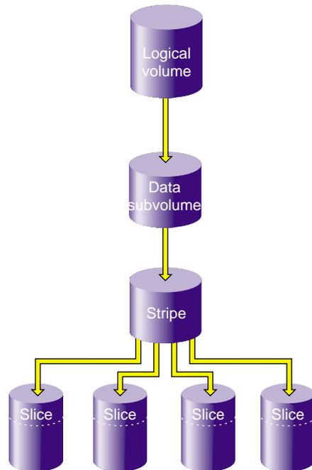
**Figure 5-2** Striping a Portion of a Disk
