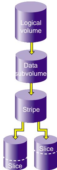
**Figure 6-28** XVM Logical Volume after Mirror Removal
