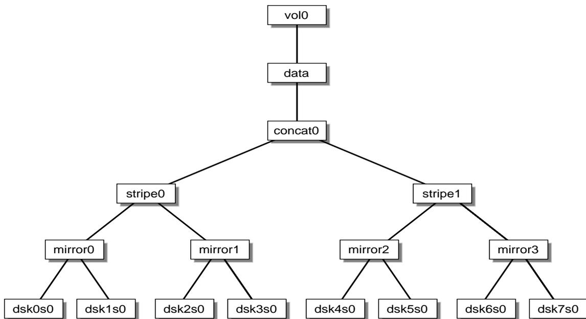
**Figure 3-1** XVM Logical Volume with System-Generated Names
