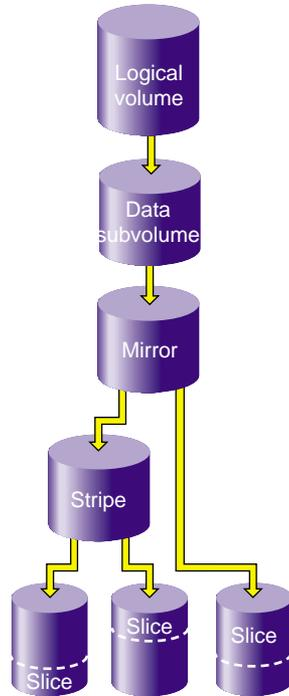
**Figure 6-27** XVM Logical Volume after Conversion from Concat to Mirror
