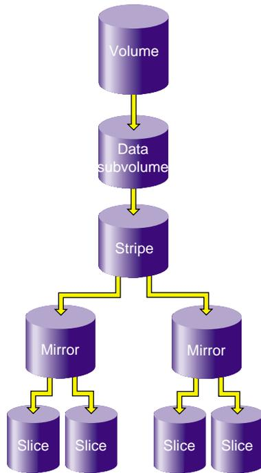
**Figure 6-5** XVM Logical Volume with Striped Mirrors
