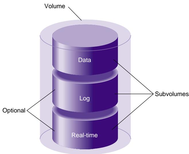
**Figure 1-8** XVM Volume with System-Defined Subvolume Types
