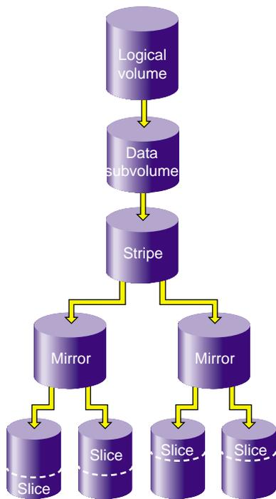
**Figure 6-29** XVM Logical Volume after Mirroring Slices
