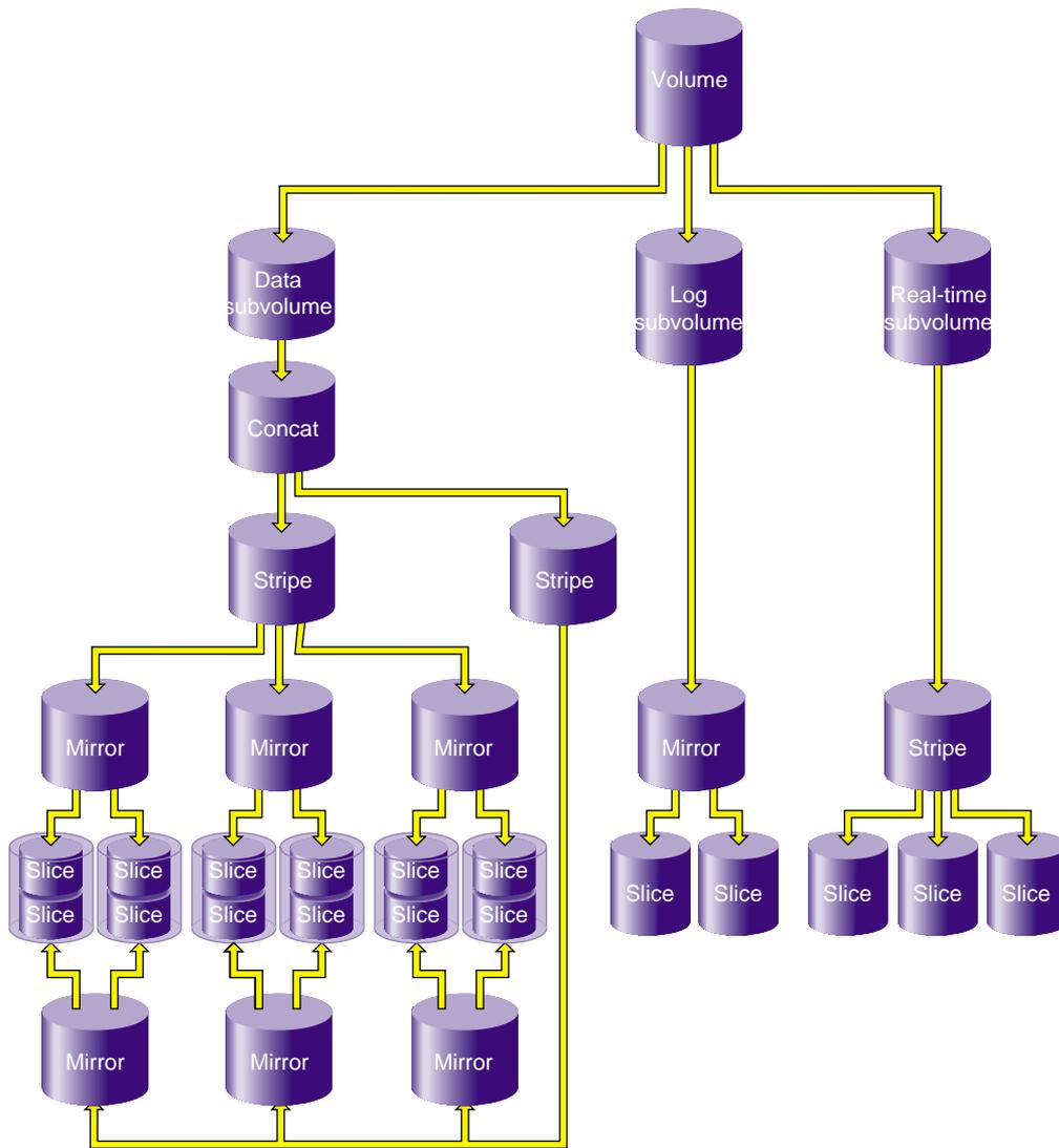
**Figure 1-7** XVM Logical Volume after Insertion of Concat
