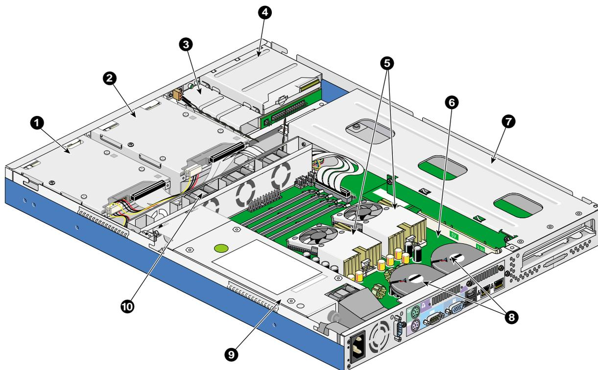
**Figure 1-4** SGI 1100 Server Internal Components
