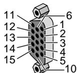
**Figure C-3** DB15 HD Port Pinout
