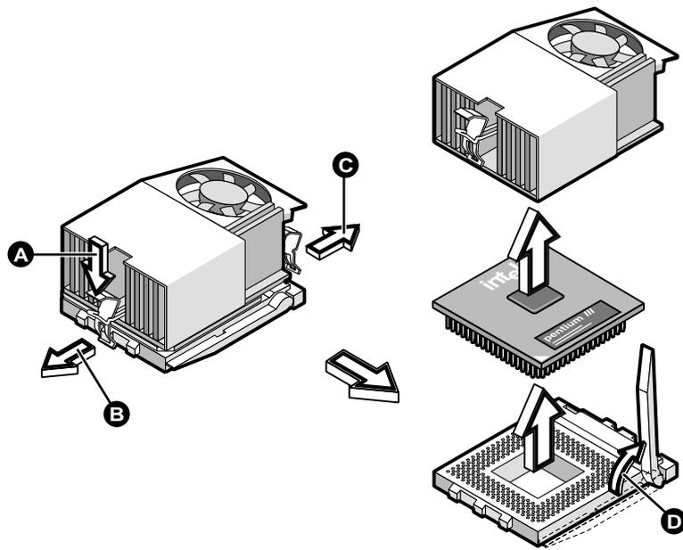
**Figure 2-48** Removing a Processor
