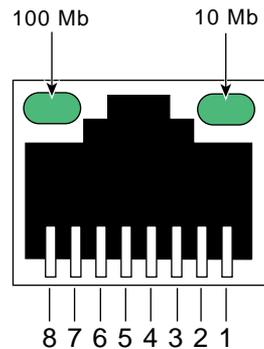
**Figure C-6** Ethernet Port Pinout
