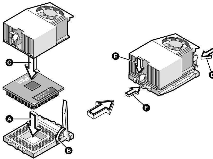
**Figure 2-49** Installing the Processor
