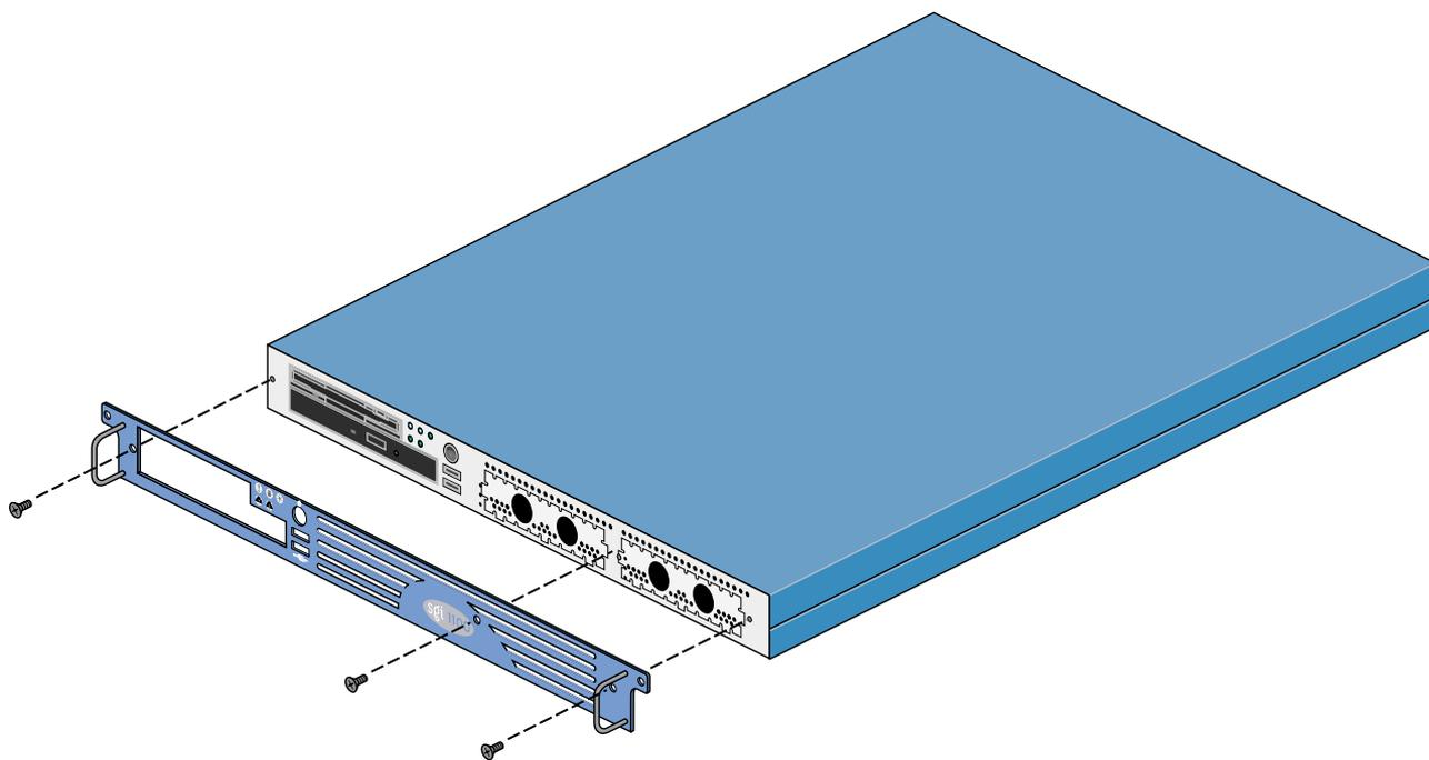
**Figure 2-3** Removing the Front Panel
