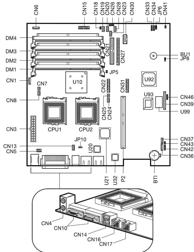
**Figure A-1** System Board Layout
