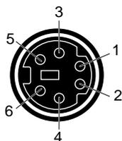
**Figure C-2** Mouse Port Pinout
