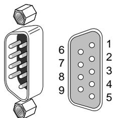
**Figure C-4** Serial Port Pinout
