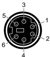
**Figure C-1** Keyboard Port Pinout
