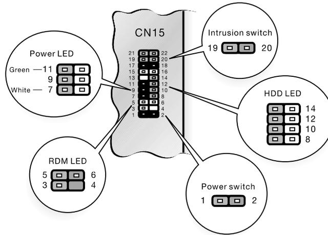
**Figure A-2** CN15 Connector Settings
