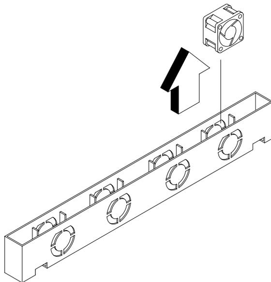
**Figure 2-12** Removing the Chassis Fan
