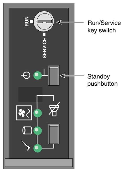
**Figure 2-3** ESI/Ops Panel: Powering On
