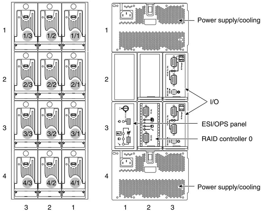
**Figure 1-8** Module Locations and Bay Numbering (Tower Configuration)
