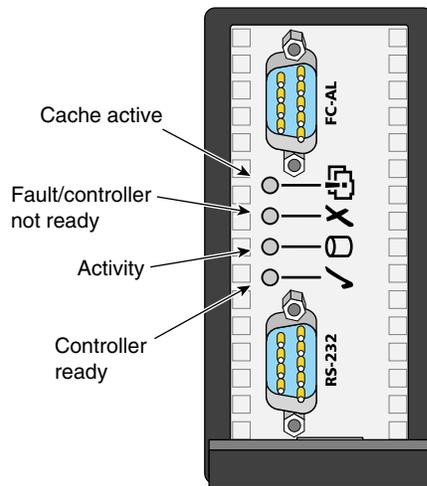
**Figure 5-4** RAID Controller Panel LEDs
