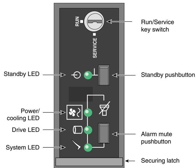
**Figure 5-1** ESI/Ops Panel Indicators and Switches
