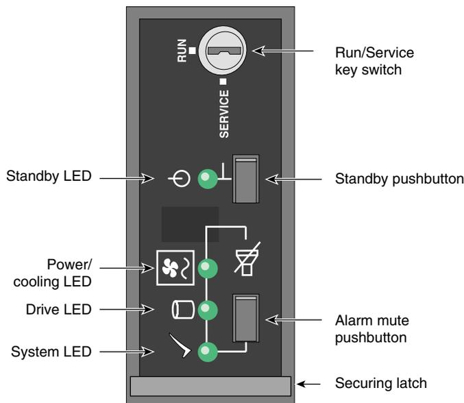
**Figure 2-4** ESI/Ops Panel Indicators and Switches
