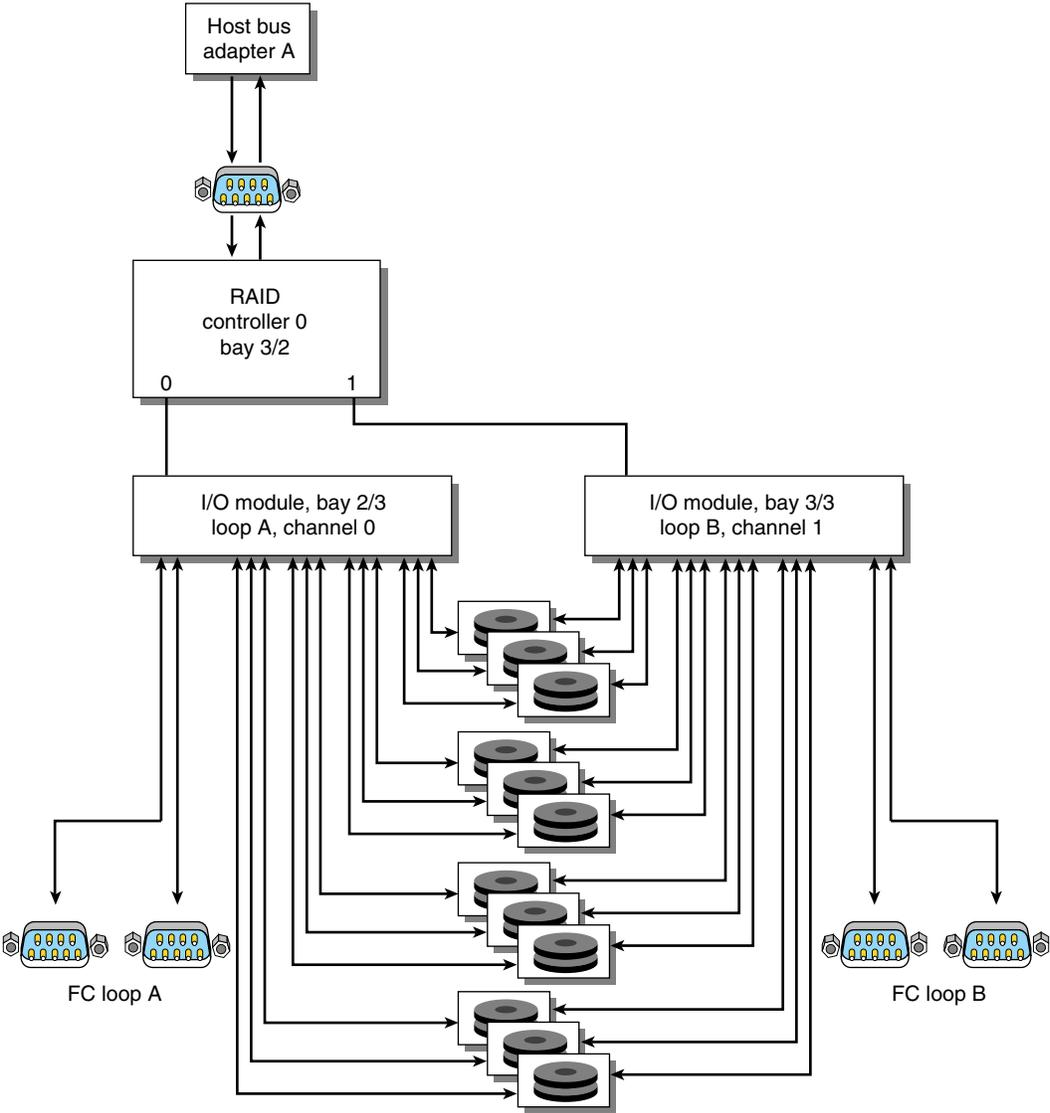
**Figure 4-3** Single-Controller/Point-to-Point/Single-Host Example
