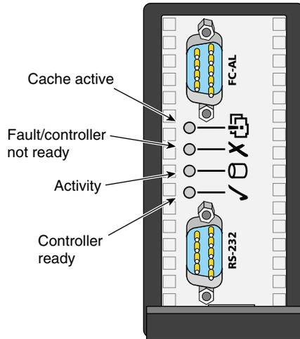
**Figure 1-5** RAID Controller Panel Features
