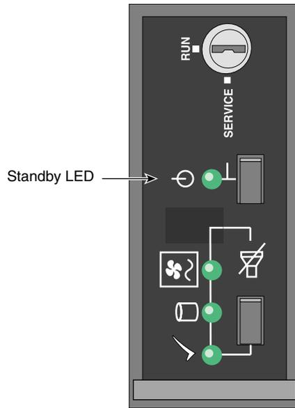
**Figure 2-2** EPI/Ops Panel: Standby LED Indicating AC Power Is Present
