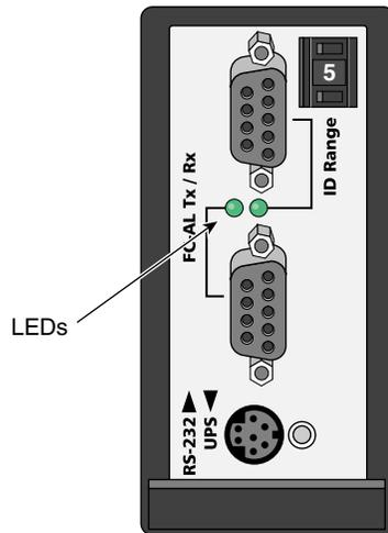
**Figure 5-3** FC LRC I/O Module LEDs
