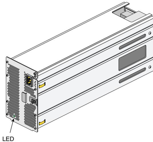
**Figure 1-3** Power Supply/Cooling Module
