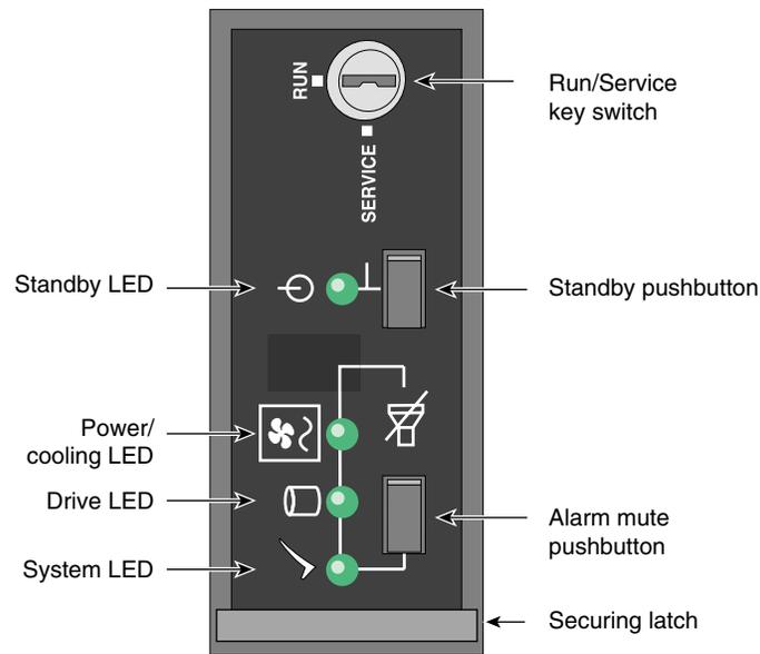
**Figure 1-4** ESI/Ops Panel Indicators and Switches
