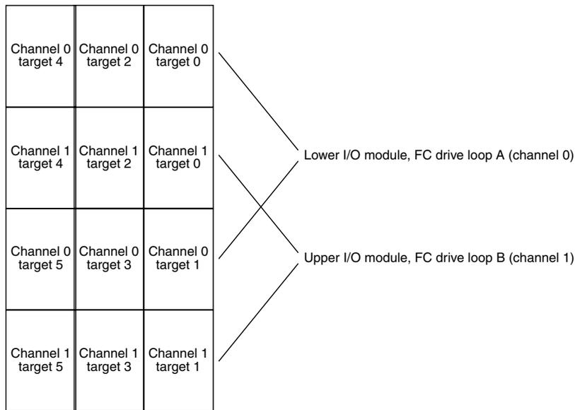
**Figure 4-2** I/O Modules, Channels, and Loops
