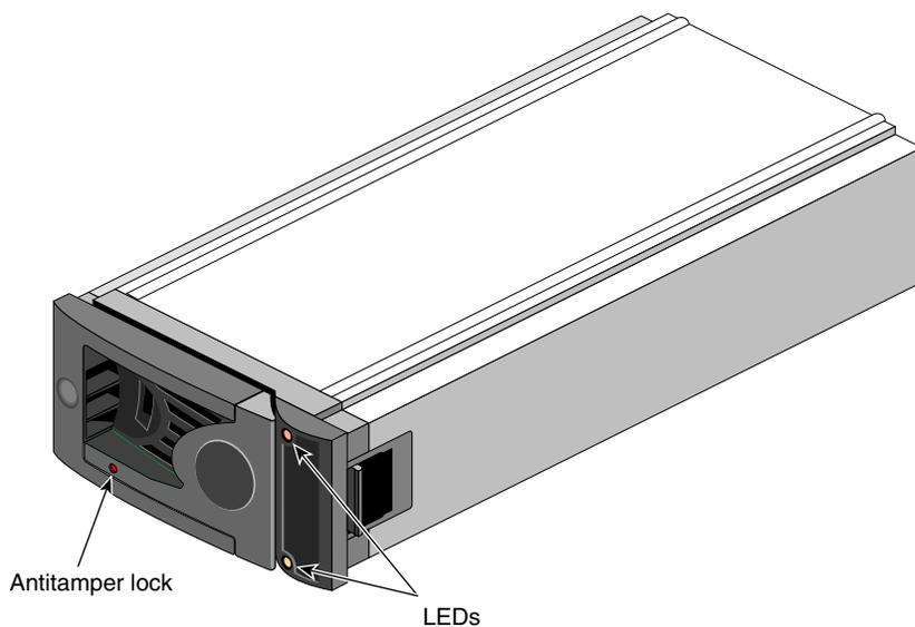
**Figure 1-7** Disk Drive Module
