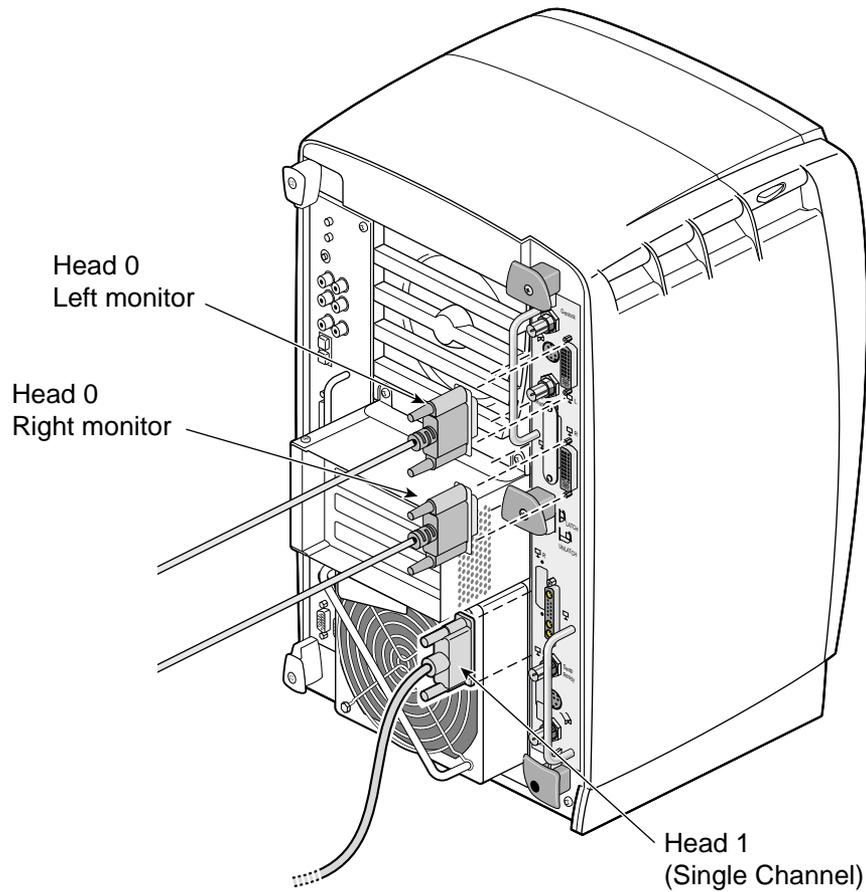
**Figure 3-3** Connecting the Monitor Signal Cables to an Upper Dual Channel Display in a Dual Head System
