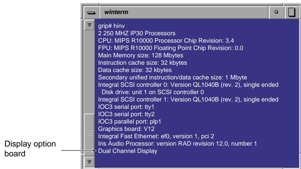
**Figure 3-6** Hardware Inventory List After Installing the Dual Channel Display
