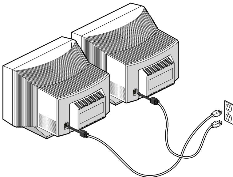
**Figure 3-5** Connecting the Power Cables
