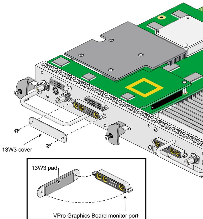
**Figure 2-26** Placing the 13W3 Cover over the VPro Graphics Board Monitor Port
