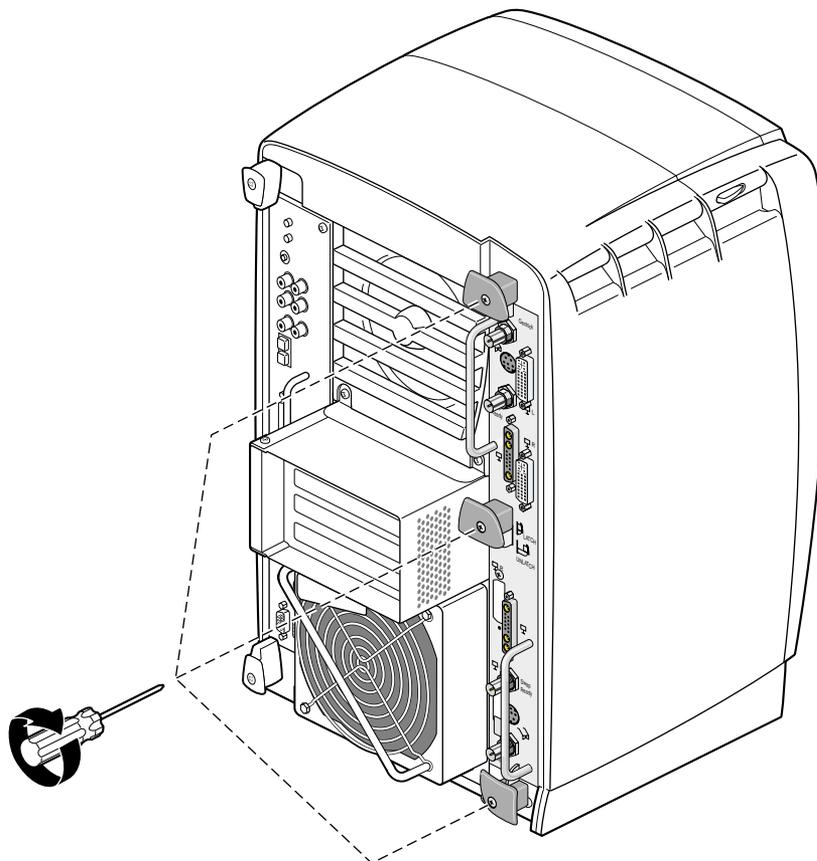
**Figure 2-31** Replacing the Dual Head XIO Module Screws
