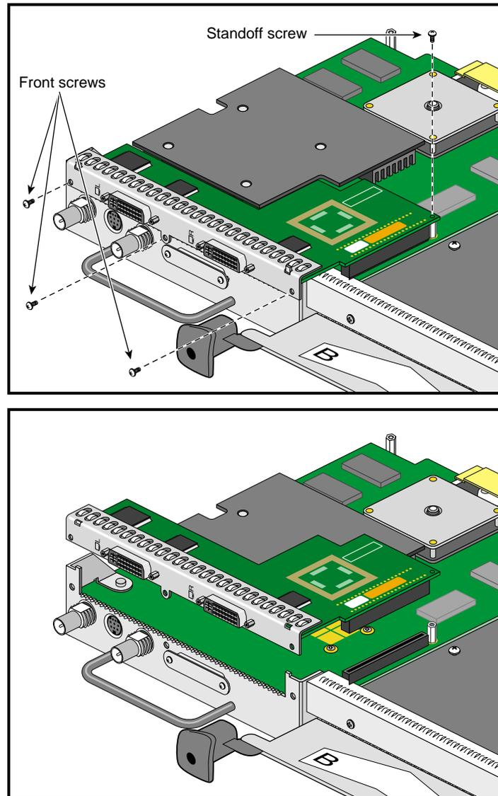
**Figure 1-24** Removing the Dual Channel Display
