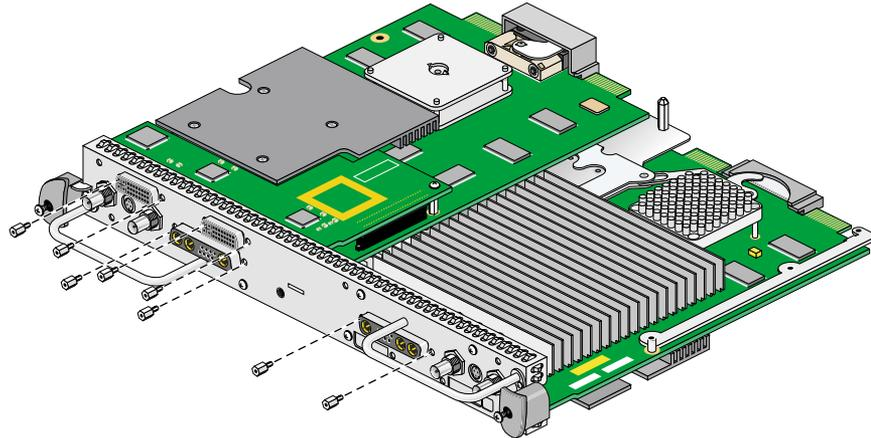
**Figure 2-36** Removing the Jackscrews from the Graphics Board I/O Panel
