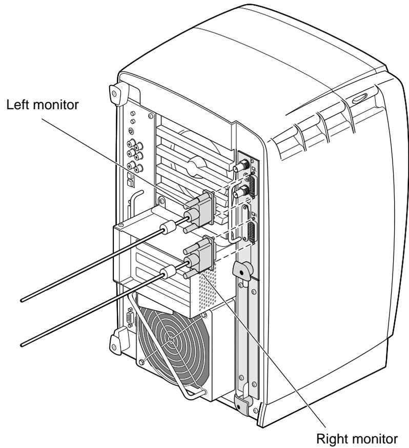
**Figure 3-2** Connecting the Monitor Signal Cables to the Dual Channel Display in a Single Head System
