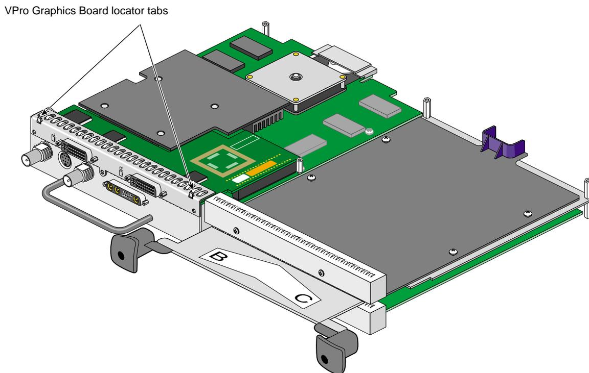
**Figure 1-17** VPro Locator Tabs Protrude through Dual Channel Display Locator Slots
