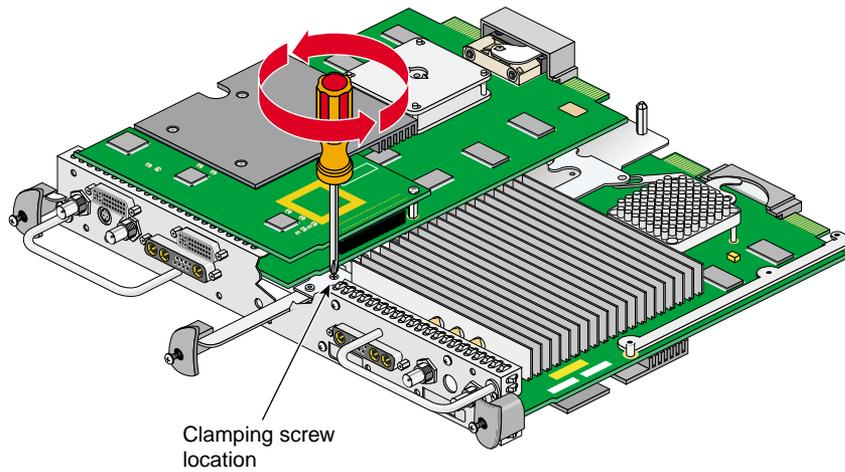
**Figure 2-33** Loosening the Center Plastic Knob Clamping Screw
