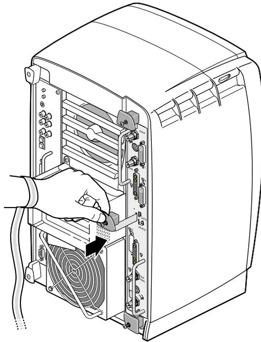
**Figure 2-30** Latching the Dual Head XIO Module
