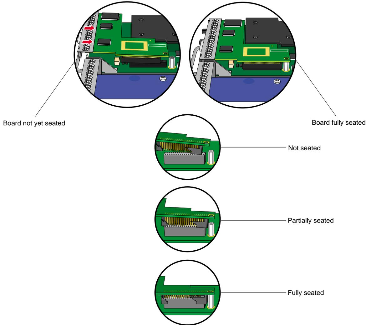
**Figure 1-16** Seating the Dual Channel Display On the VPro Graphics Board (side view)
