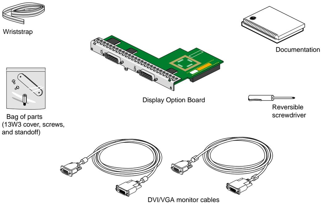
**Figure 1-1** Dual Channel Display Shipment Components
