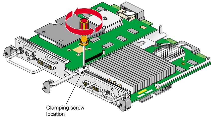
**Figure 2-11** Loosening the Center Plastic Knob Clamping Screw
