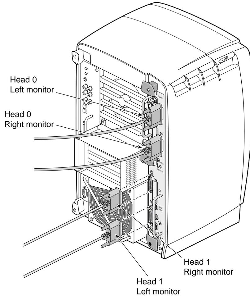
**Figure 3-4** Connecting the Monitor Cables to a Lower Dual Channel Display in a Dual Head System
