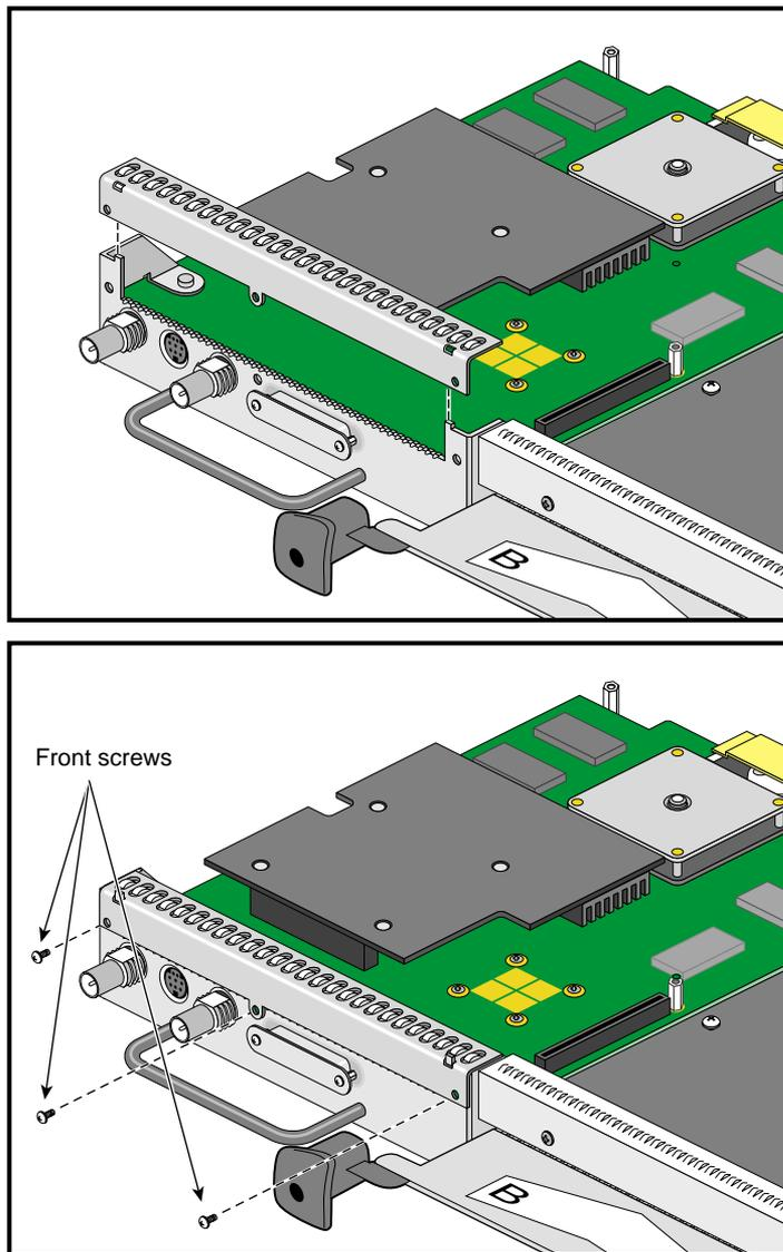
**Figure 1-25** Reinstalling the VPro Graphics Board Blank Panel
