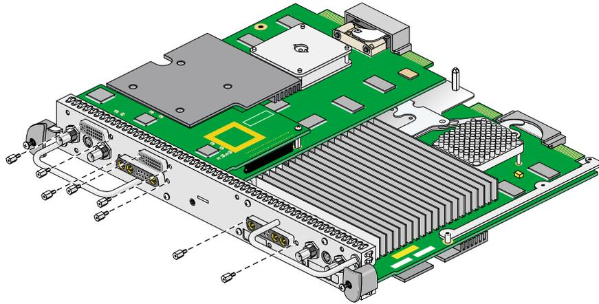
**Figure 2-23** Installing the Jackscrews on the Graphics Board I/O Panel
