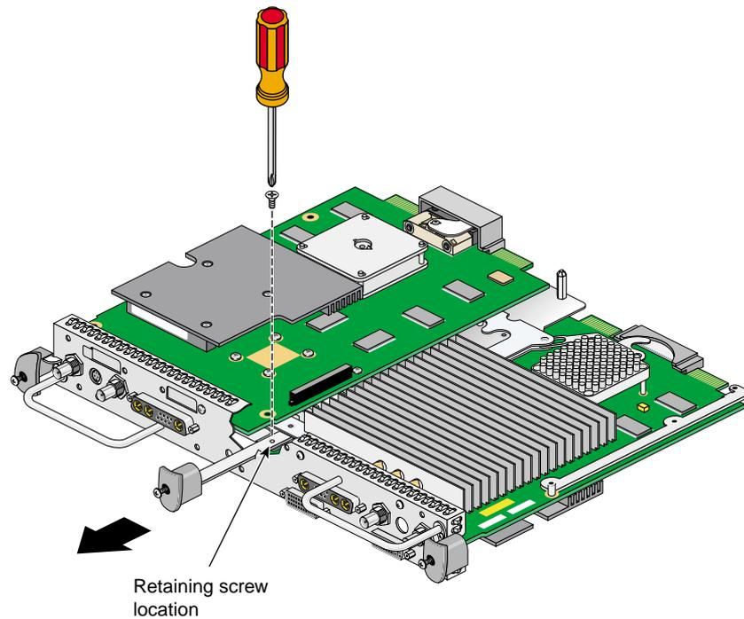
**Figure 2-34** Removing the Center Plastic Knob Retaining Screw
