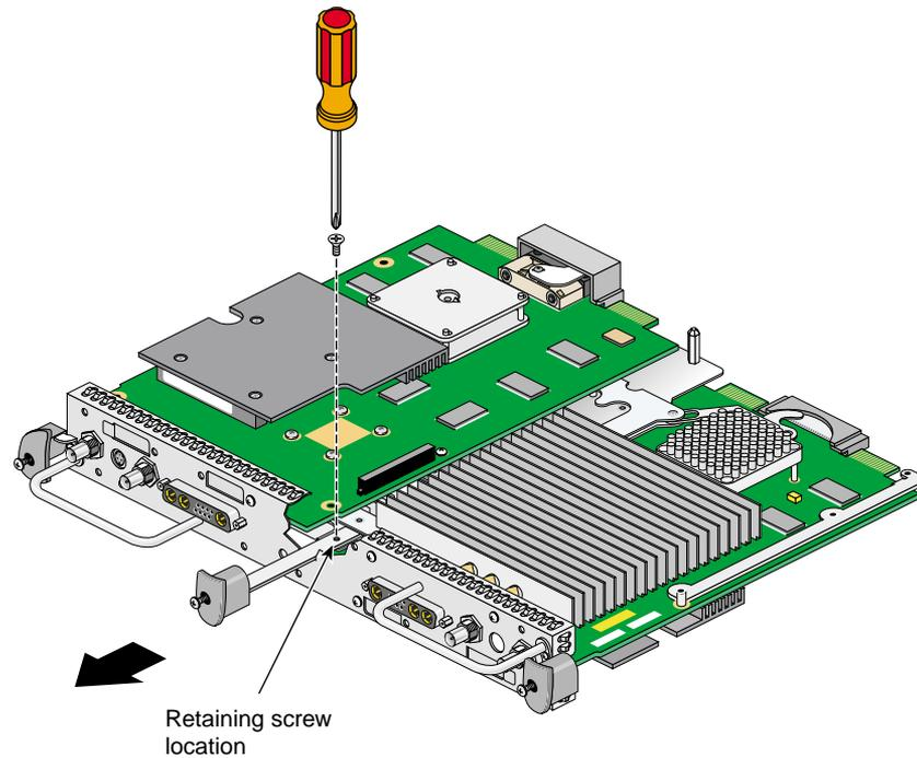
**Figure 2-12** Removing the Center Plastic Knob Retaining Screw
