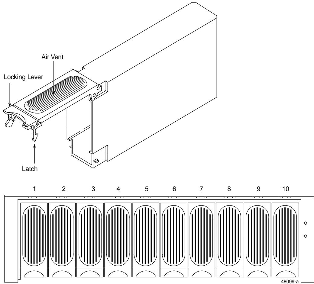
**Figure 5-4** Drive Sleds and Drive Numbering
