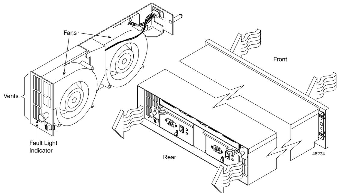
**Figure 5-5** Fan Canister and Drive Enclosure Air Flow
