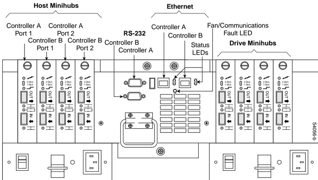
**Figure 2-3** TP9400 Interface Components
