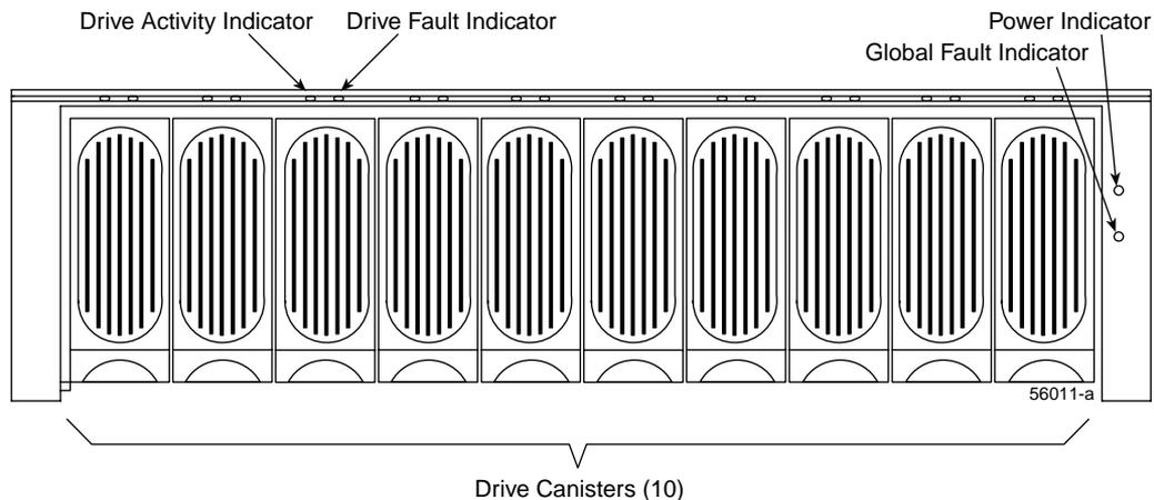
**Figure 5-1** Front View of the Drive Enclosure
