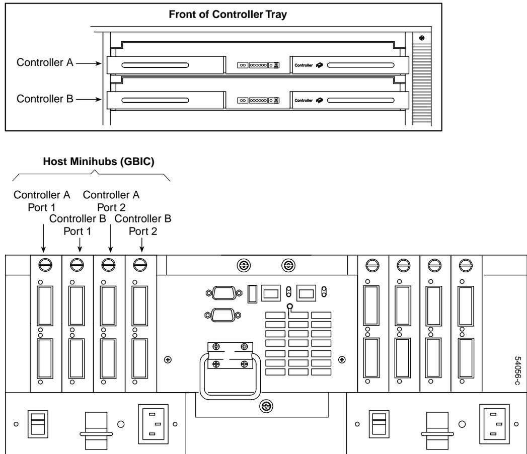
**Figure 2-14** Controller Enclosure Host Interface Connectors
