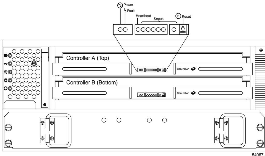
**Figure 2-6** Redundant Controllers and Indicator Lights
