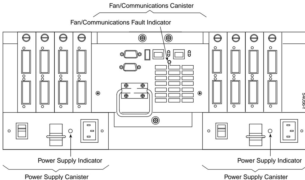
**Figure 3-3** Fan/Communications and Power Supply Indicators (Rear)
