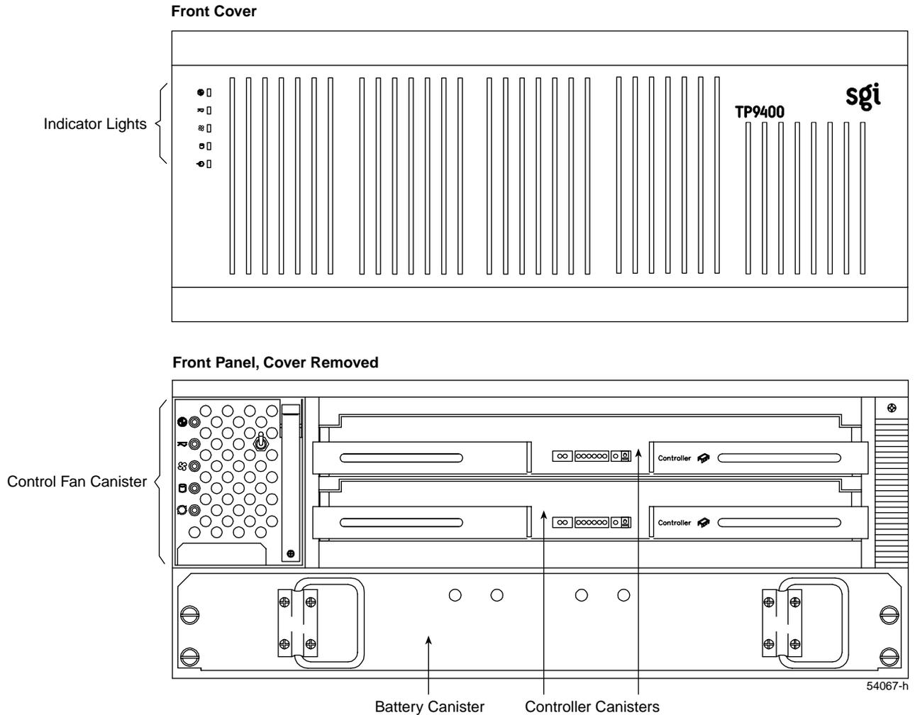
**Figure 2-1** Front View of the Controller Enclosure
