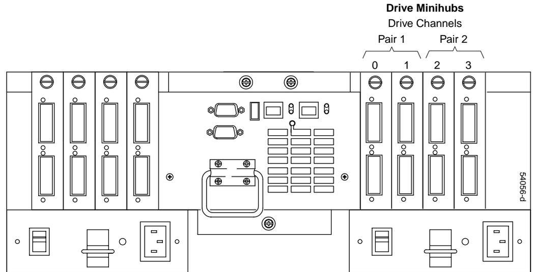
**Figure 2-15** Controller Enclosure Drive Minihub Connectors (Rear)
