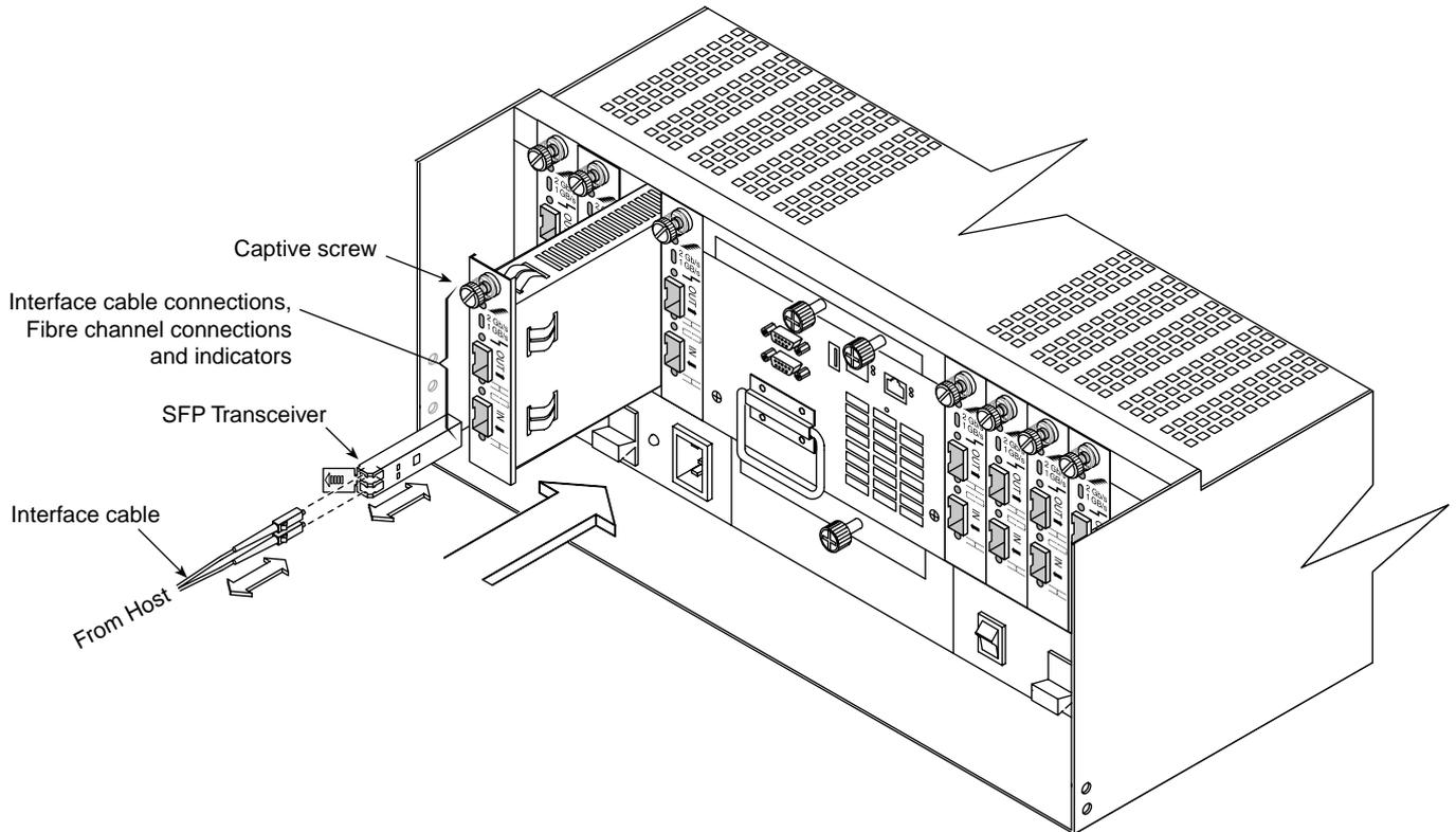
**Figure 2-17** Removing and Installing an SFP Transceiver
