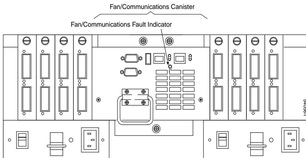
**Figure 2-10** Fan/Communications Canister and Fault Indicator
