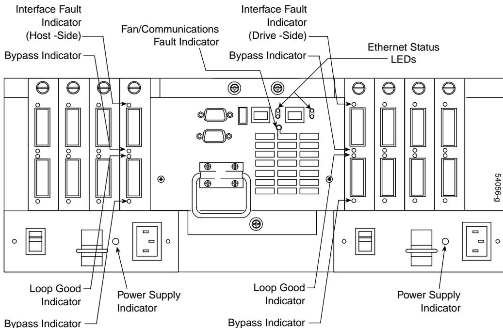
**Figure 3-6** 1 GB Interface Controller Rear Indicator Lights (GBIC)
