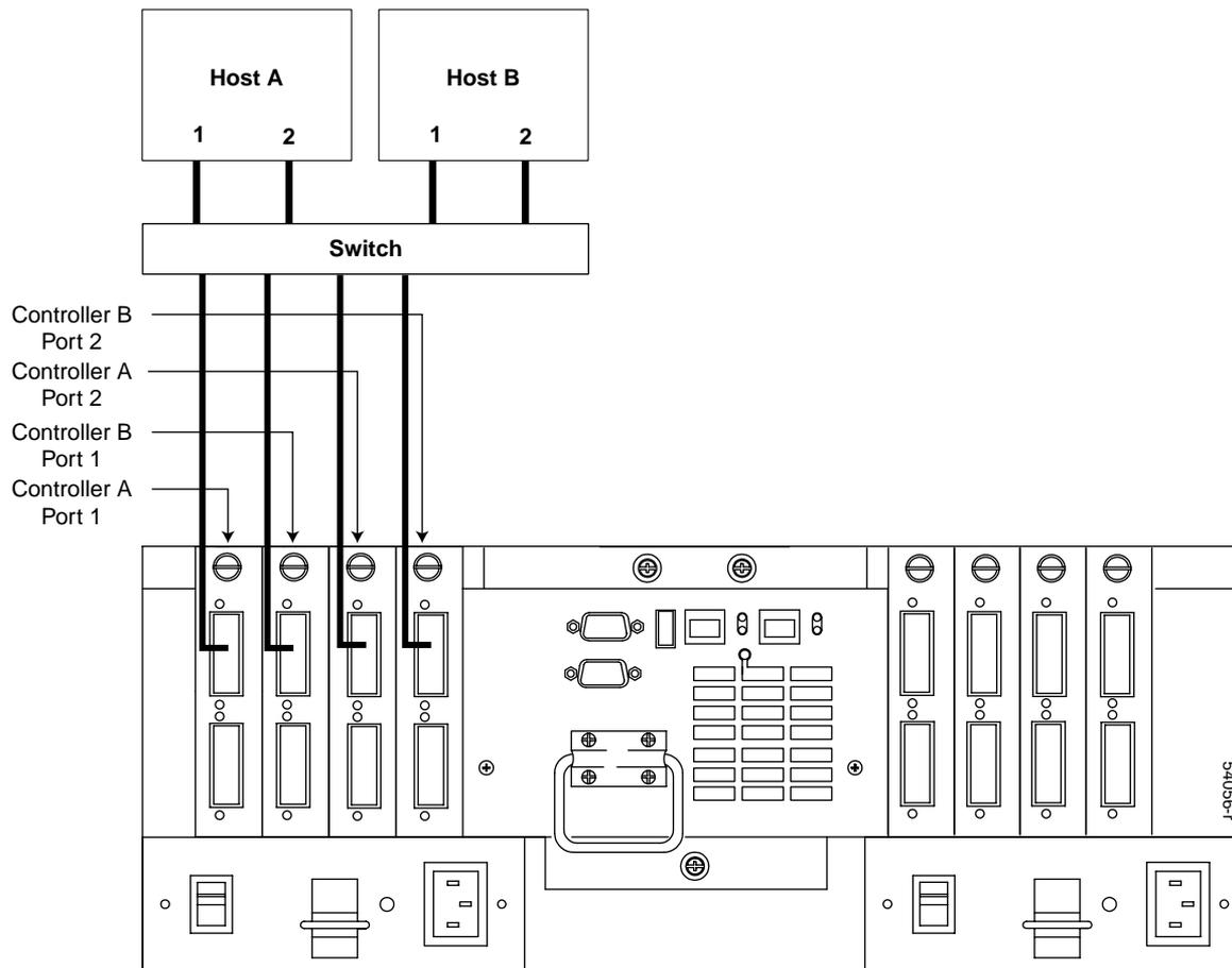
**Figure 8-11** Switch Connect — 2 Host - 2 HBA/Host
