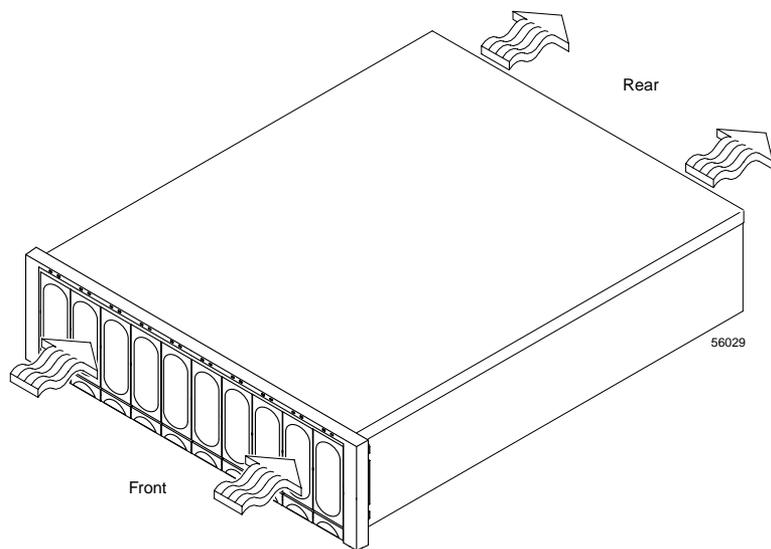
**Figure A-9** Drive Enclosure Air Flow
