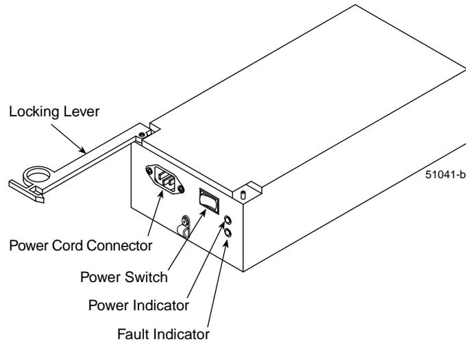
**Figure 5-7** Power Supply Canister
