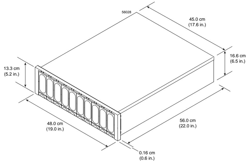
**Figure A-8** Drive Enclosure Dimensions
