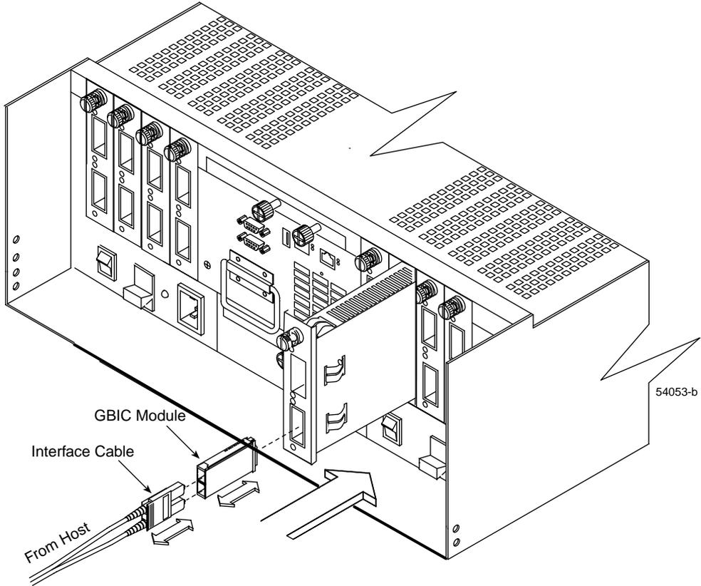
Figure 2-4 GBIC Minihub with GBIC Module
