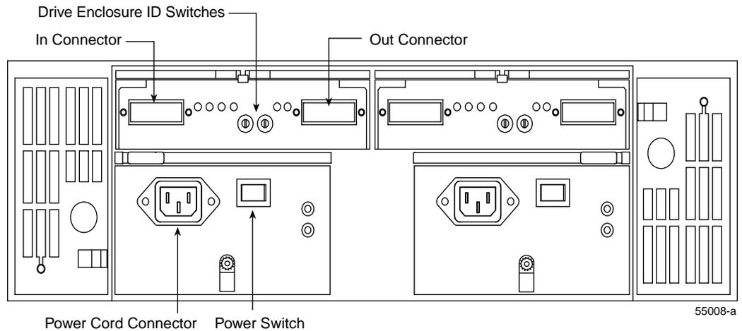
**Figure 5-3** Connectors and Switches (Rear)
