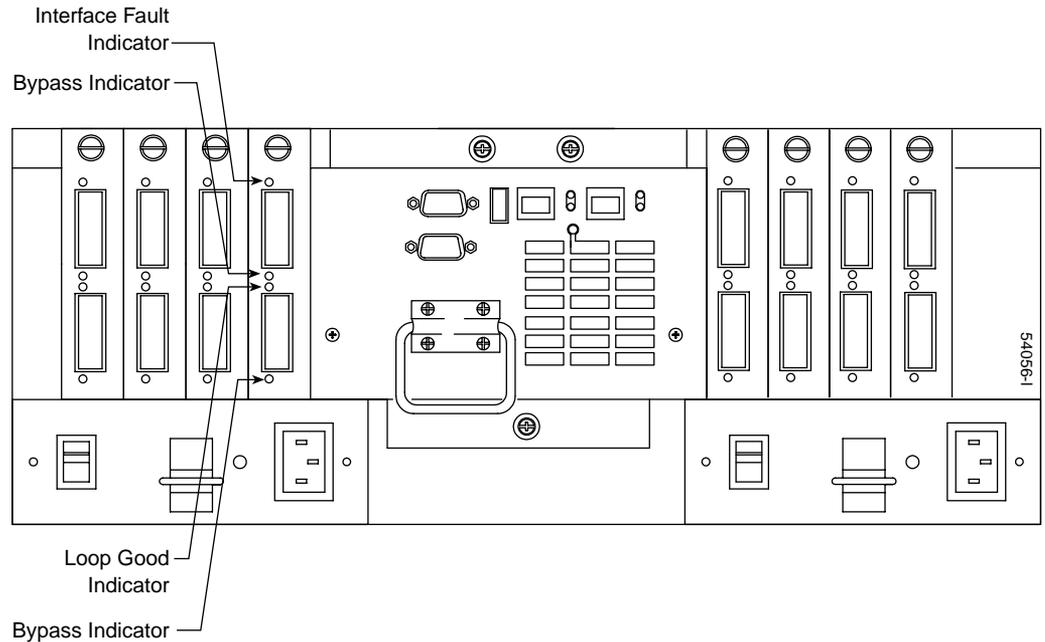
**Figure 2-13** Minihub Canister and indicator lights
