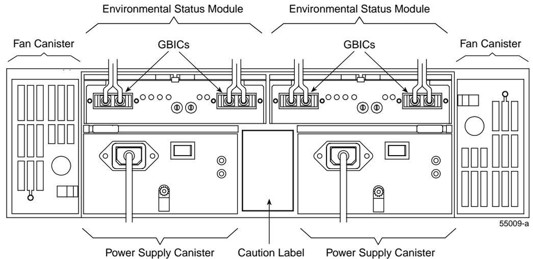
**Figure 5-2** Rear View of the Drive Enclosure
