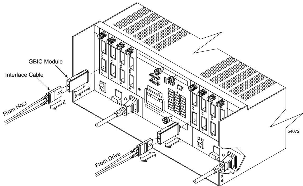
**Figure 2-16** Removing and Installing a GBIC Module
