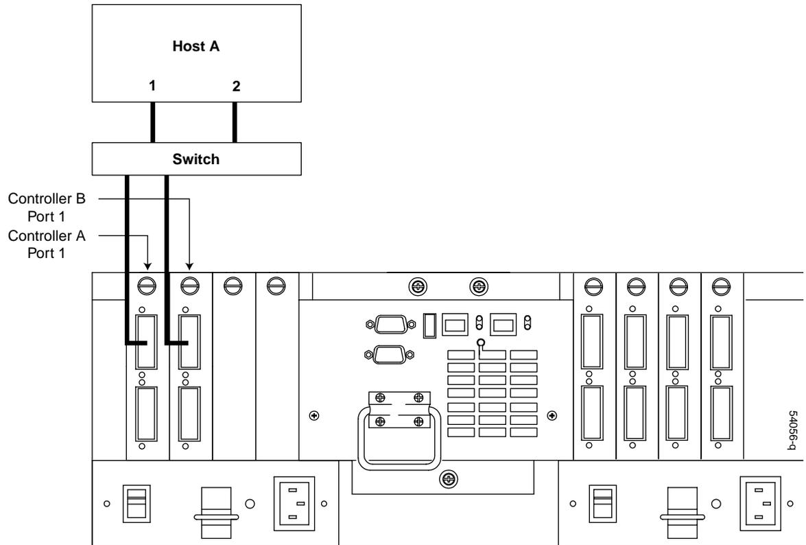
**Figure 8-10** Switch Connect — 1 Host - 2 HBA
