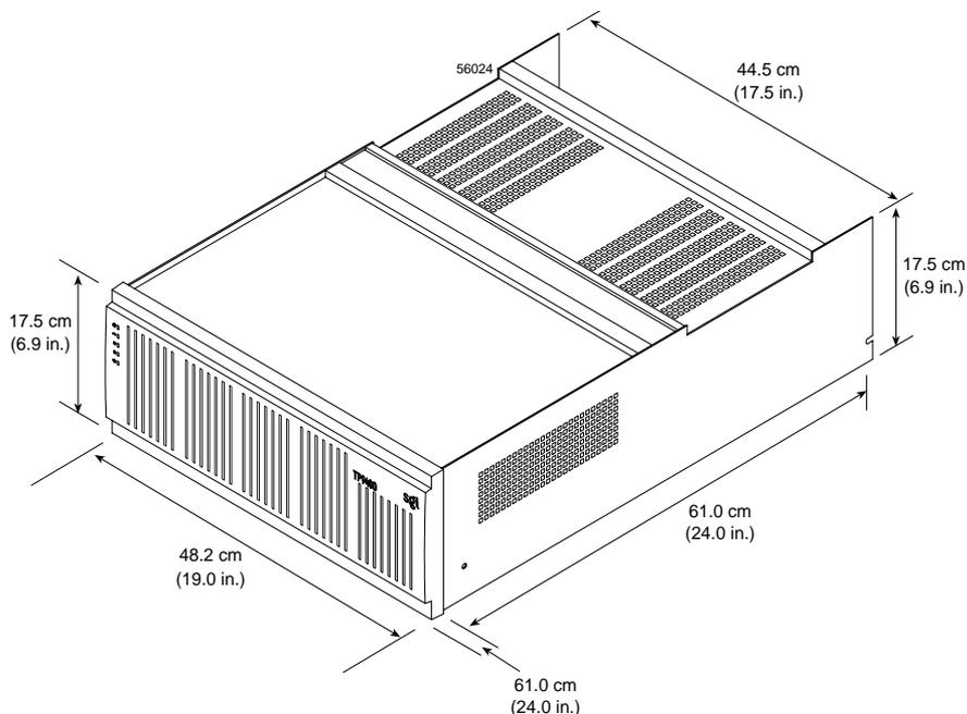
**Figure A-6** Controller Enclosure Dimensions
