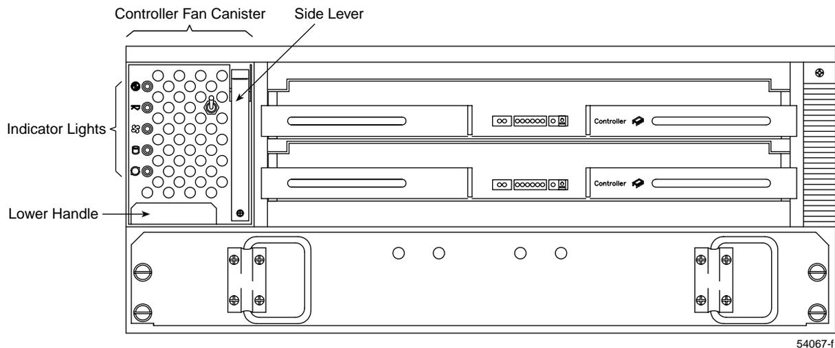
**Figure 2-8** Controller Fan Canister
