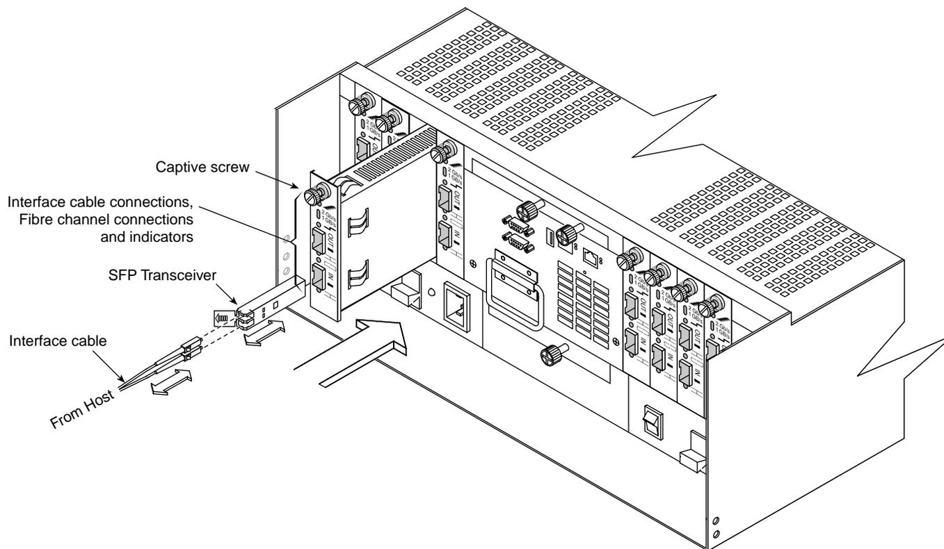
**Figure 2-5** SFP Minihub with SFP Transceiver
