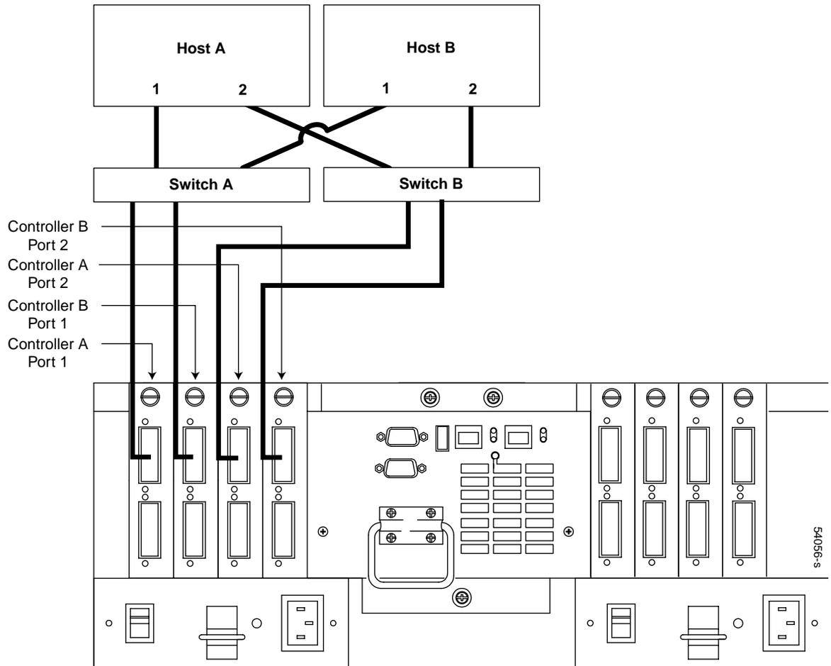
**Figure 8-12** Multi-Switch Connect — 2 Host
