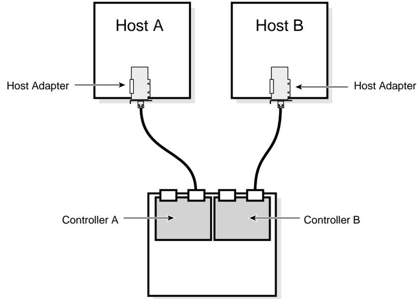
**Figure 8-8** Direct Host Connect for Non fail-over Configuration
