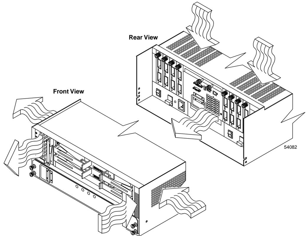
**Figure 2-9** Controller Enclosure Air Flow
