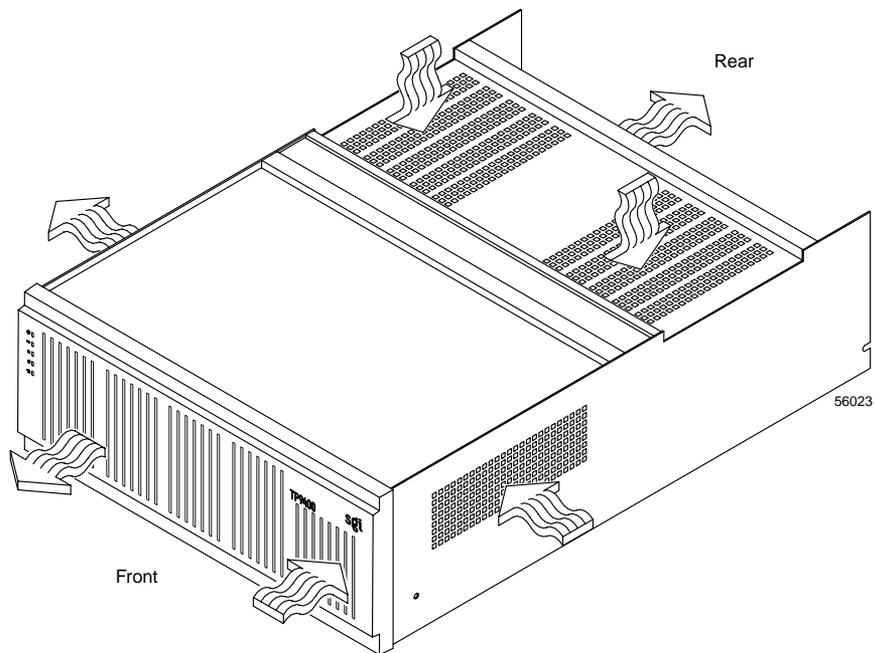
**Figure A-7** Controller Enclosure Air Flow
