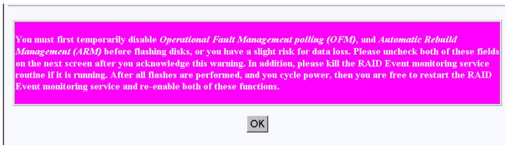
**Figure 3-80** Flash New Firmware Onto Selected IBM and Seagate Disk(s)
