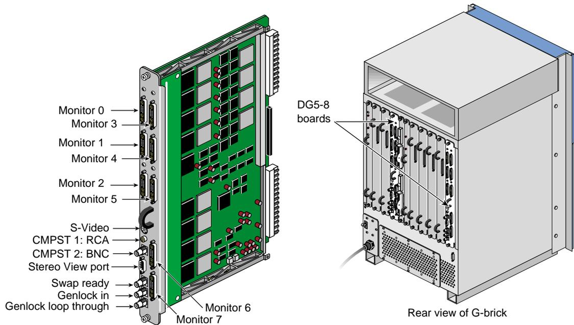
**Figure 13-8** DG5 (Display Generator) Board
