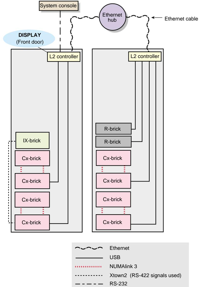
**Figure 1-1** Connecting System Console to Multiple L2 Controllers
