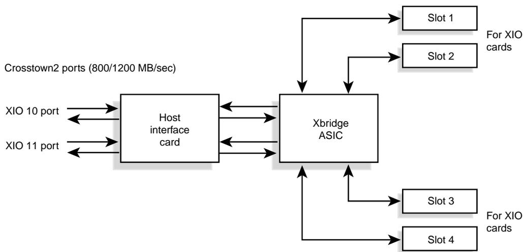
**Figure 6-1** X-brick Block Diagram
