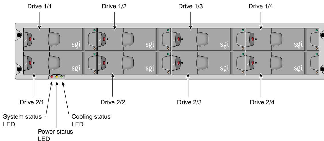
**Figure 10-1** Front View of TP900 Storage Module
