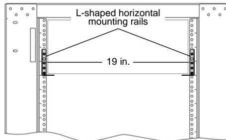
**Figure 2-3** L-shaped Mounting Rails
