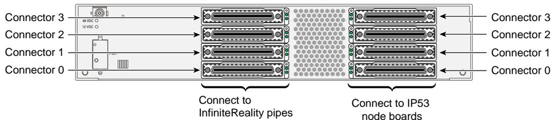
**Figure 13-10** Rear View of N-Brick
