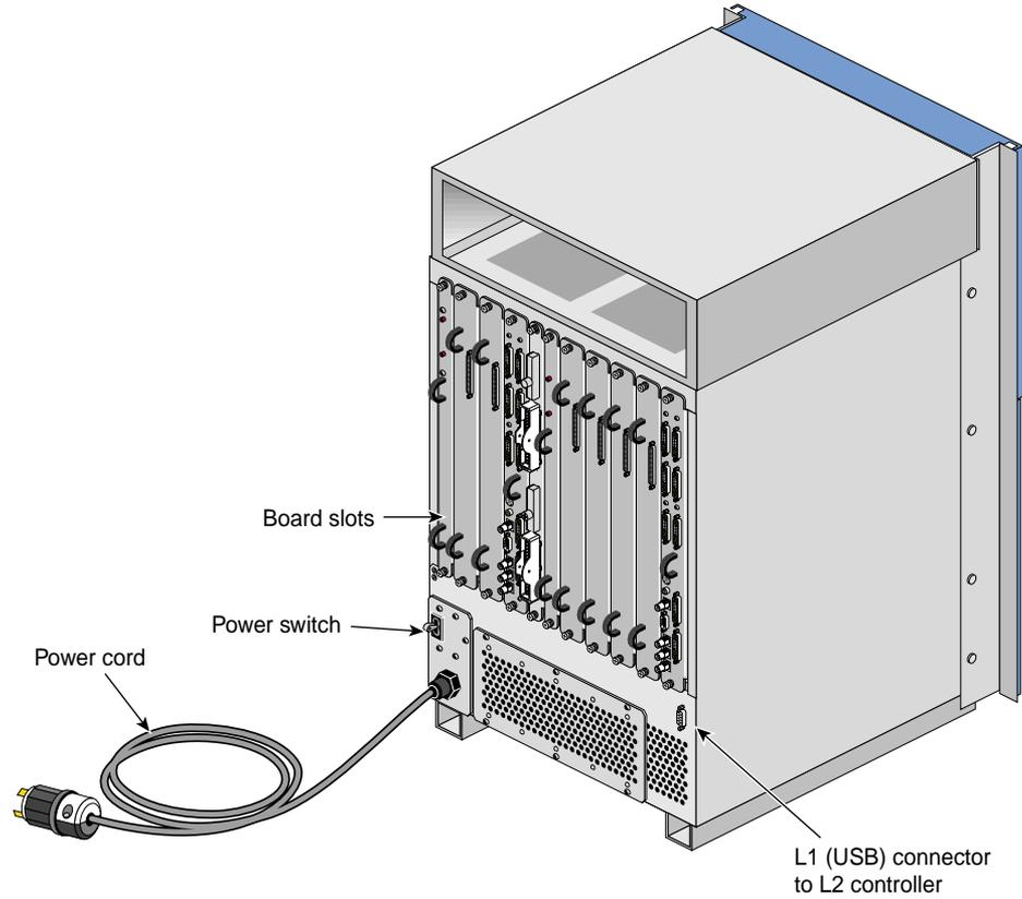
**Figure 13-3** Rear View of G-brick
