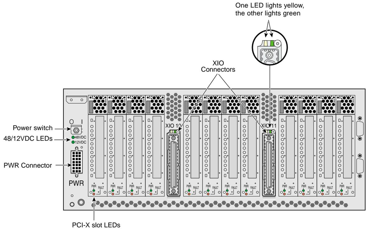
**Figure 5-4** Rear Panel of PX-brick
