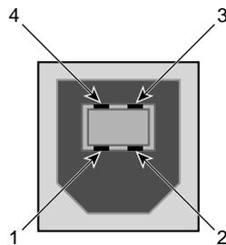
**Figure A-1** USB Type B Connector
