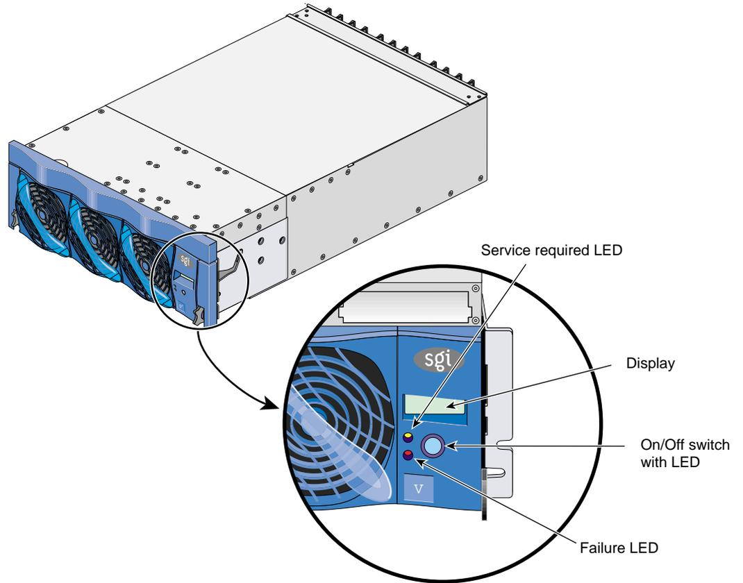
**Figure 12-2** Front View of V-Brick
