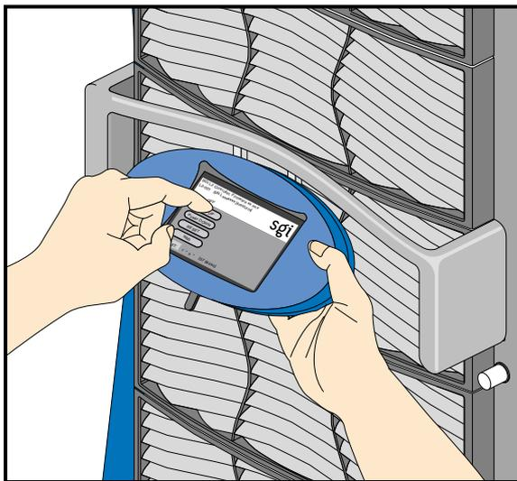
**Figure 1-5** L2 Controller Touch Display
