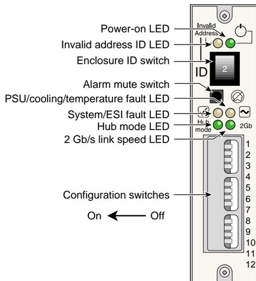
**Figure 11-6** Operator's Panel
