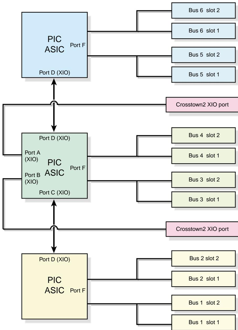
**Figure 5-2** PX-brick Block Diagram
