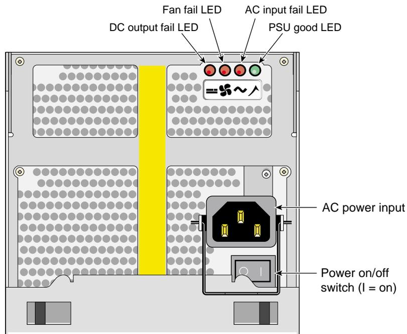
**Figure 11-5** Power Supply/Cooling Module
