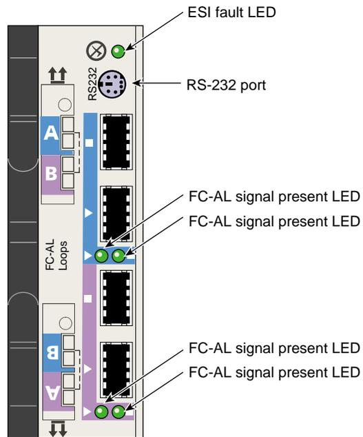
**Figure 11-7** D-brick2 Loop Resiliency Circuit (LRC) Module
