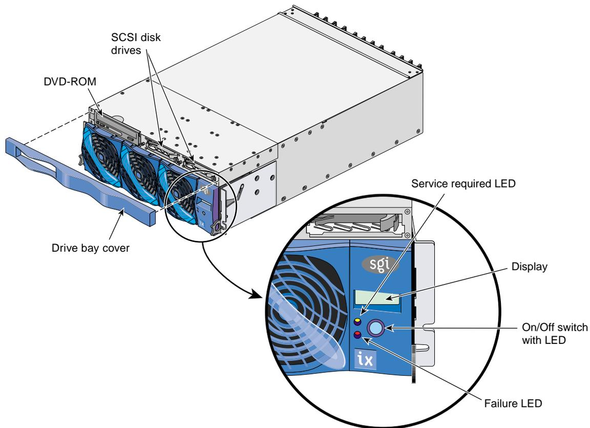
**Figure 4-4** Front Panel of IX-brick
