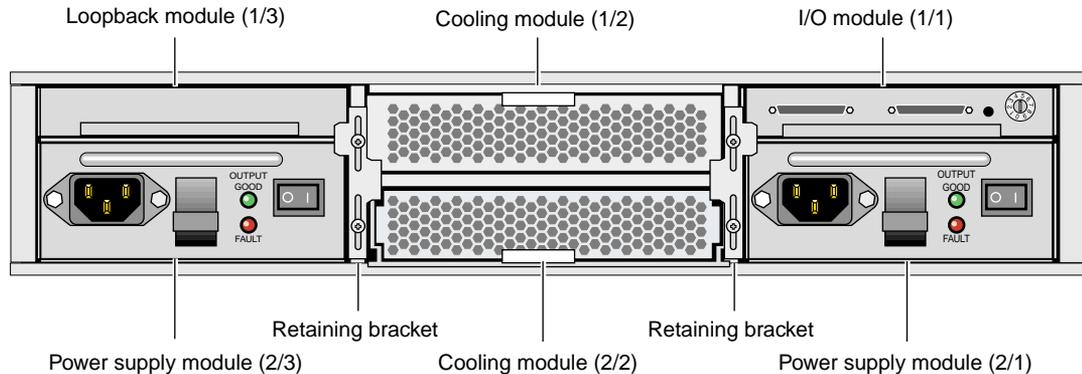
**Figure 10-3** Rear View of TP900 Storage Module
