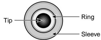
**Figure A-5** Stereo Jack Connector Conductors
