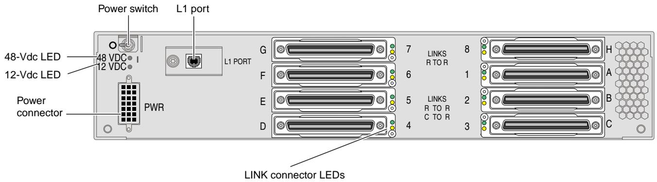
**Figure 7-4** Rear View of R-Brick
