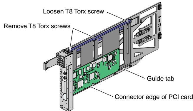
**Figure 14-5** Mounting Half-height Card in Carrier
