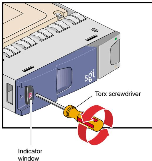
**Figure 14-16** Unlocking Drive Carrier Module
