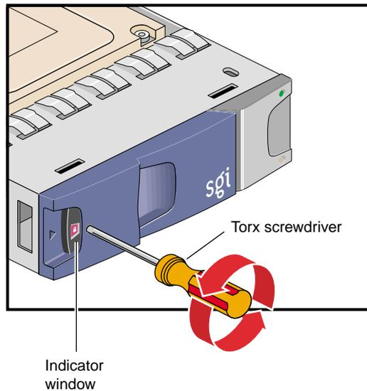
**Figure 14-15** Unlocking Anti-Tamper Lock
