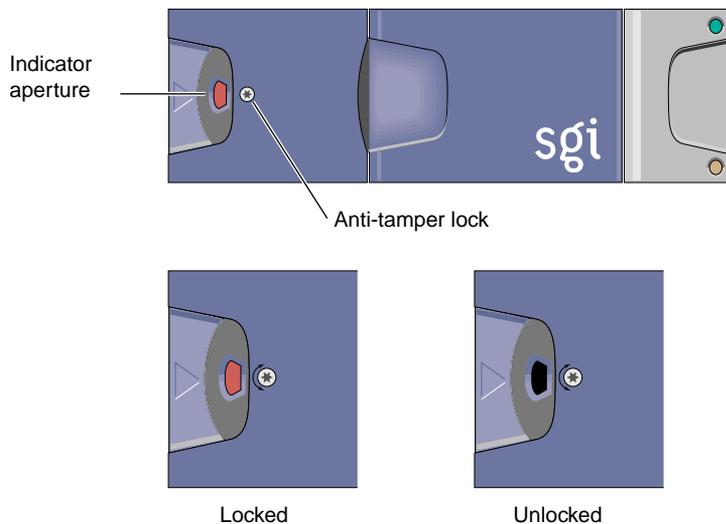
**Figure 11-3** Anti-Tamper Locking on D-brick2 Disk Drive
