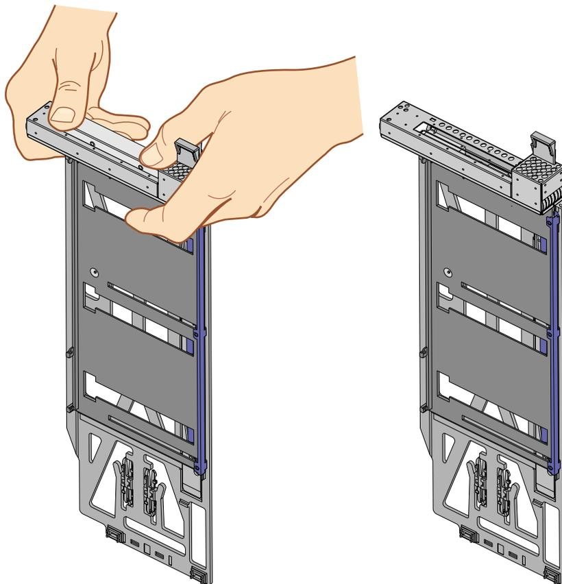
**Figure 14-2** Extracting Carrier Metal Filler Plate
