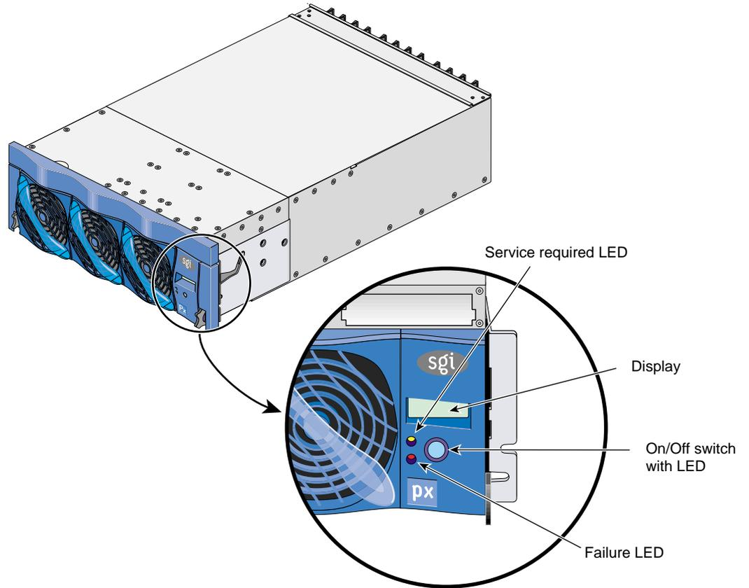
**Figure 5-3** Front Panel of PX-brick
