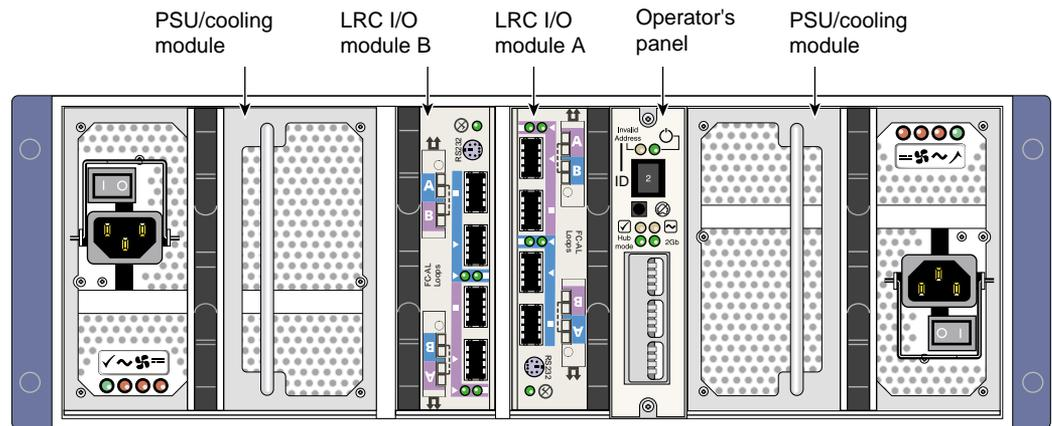
**Figure 11-4** Rear View of D-brick2
