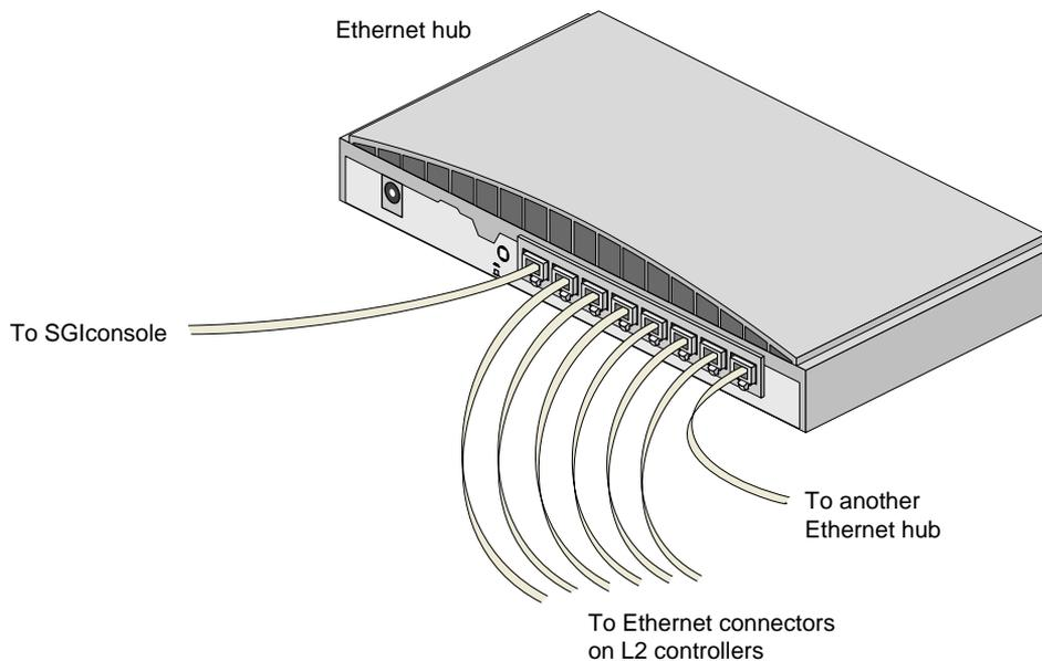
**Figure 8-4** Ethernet Hub Connections (Example)
