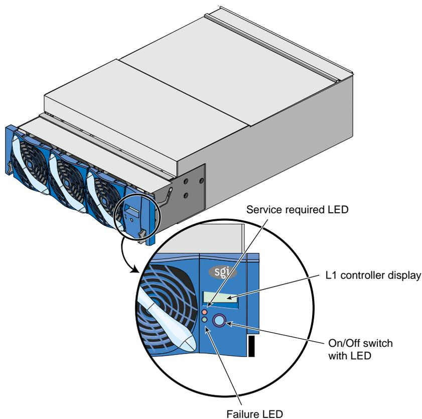
**Figure 6-2** Front Panel of X-brick
