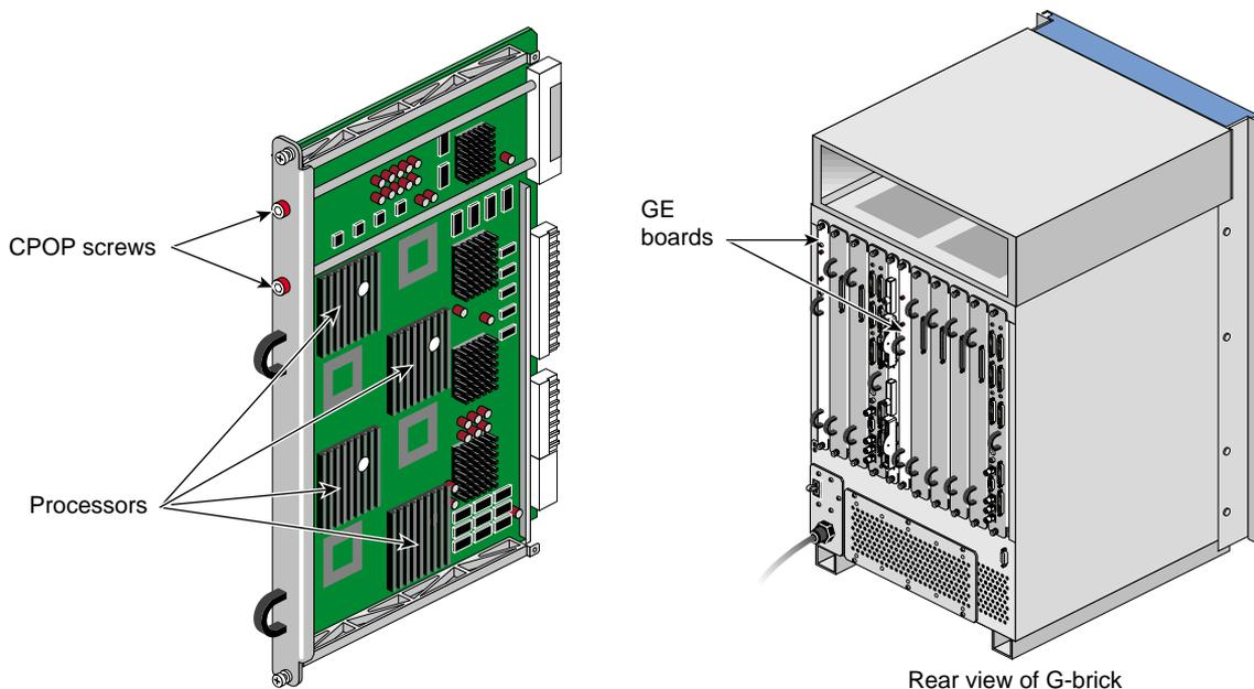
**Figure 13-6** GE (Geometry Engine) Board
