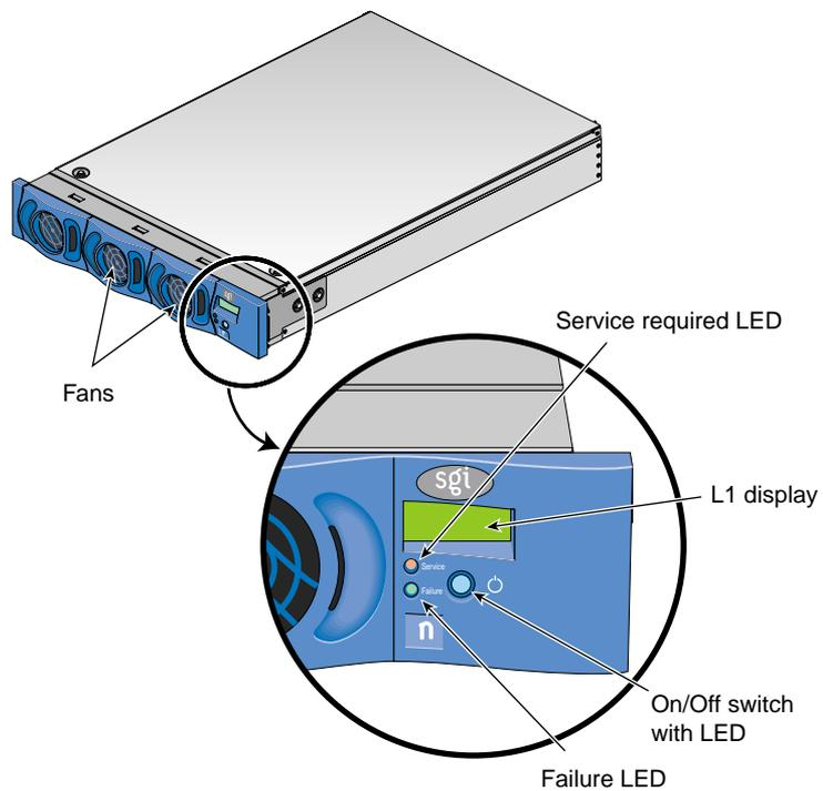
**Figure 13-9** Front View of N-Brick
