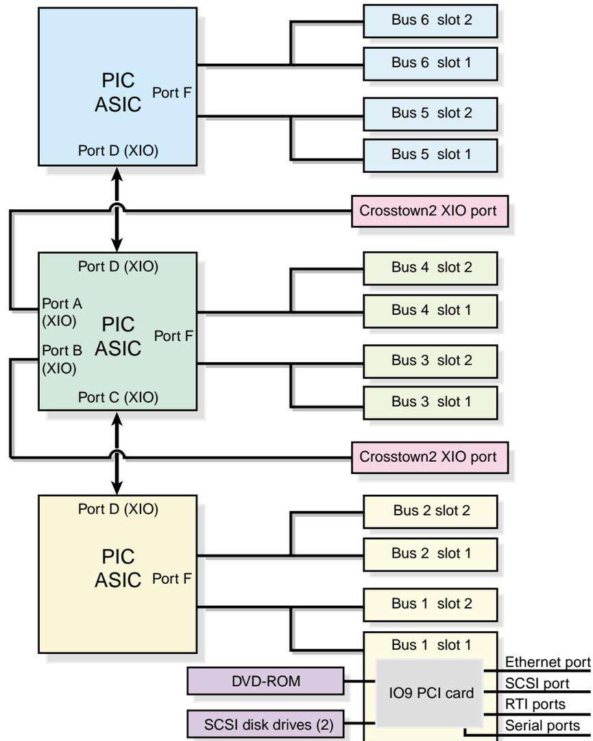
**Figure 4-2** IX-brick Block Diagram
