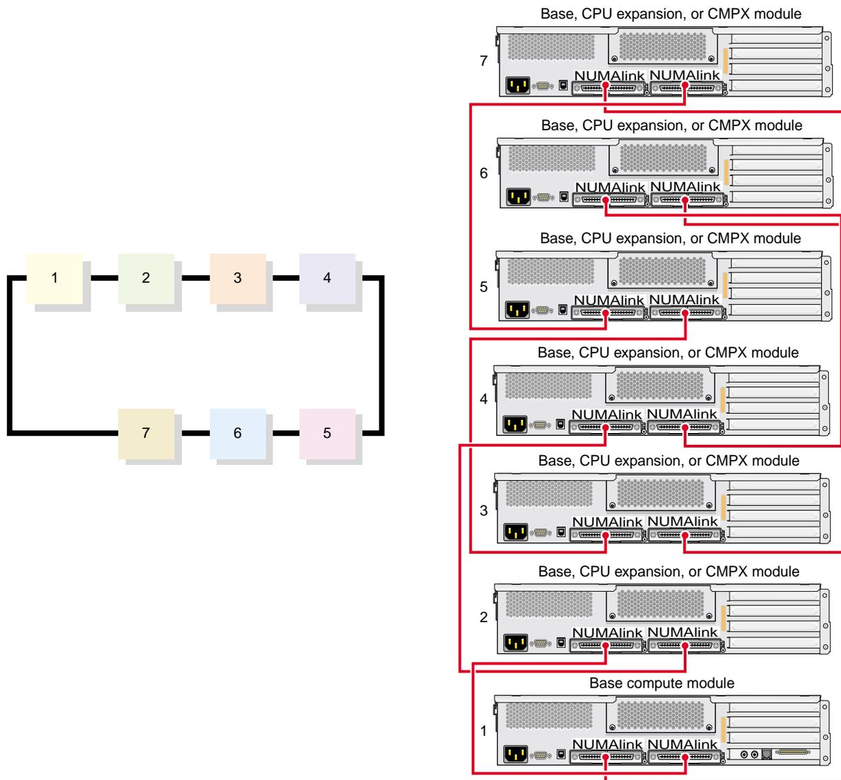
Figure 2-9 Seven Module Ring Topology
